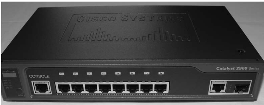
FIGURE 5.9 Typical Ethernet switch
