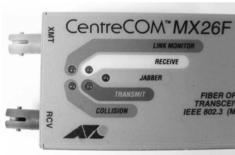
FIGURE 5.5 A 100Base-TX to 100Base-FX transceiver
