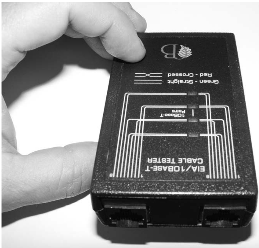
FIGURE 18.6 An inexpensive cable tester
