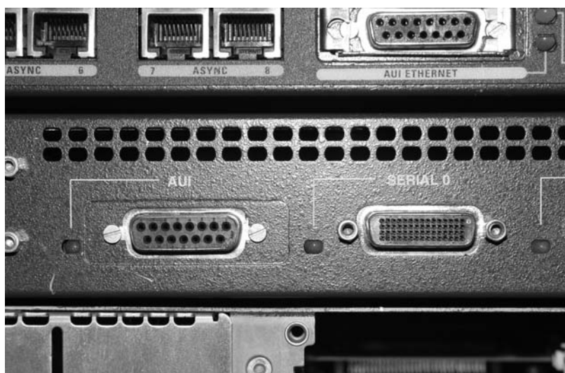
FIGURE 5.6 Router with a DIX (AUI) connector
