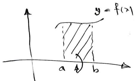
$$y = f(x) \quad [a, b] \quad V = \pi \int_a^b f^r(x) dx$$
