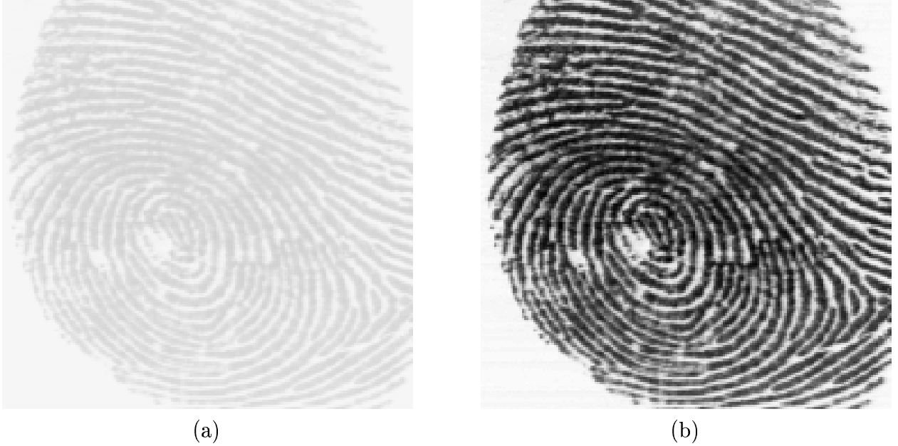
Figure 5: The result of normalization; (a) input image; (b) normalized image ( M_0 = 100, VAR_0 = 100 ).
