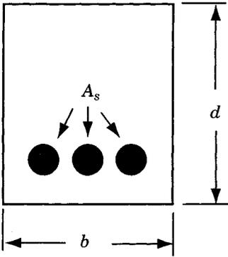
**Figure 1.12** Cross section of a reinforced concrete beam.
