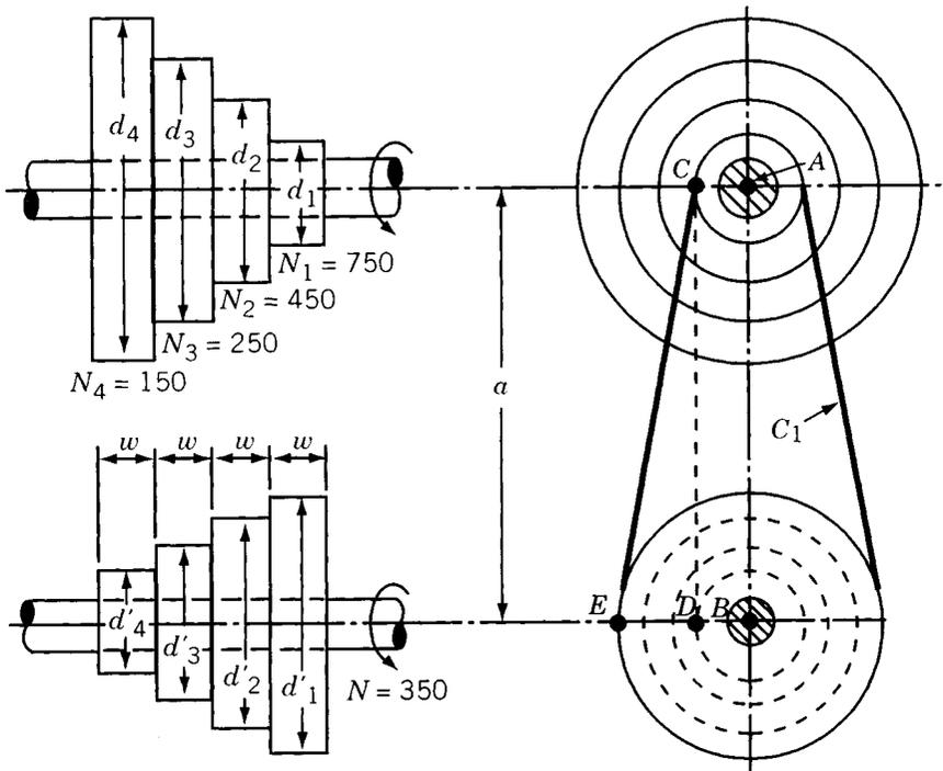
Figure 1.9 Step-cone pulley.
