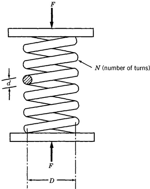
Figure 1.10 Helical spring.
