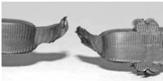
(b) Ductile Rupture Outside Fusion Interface
