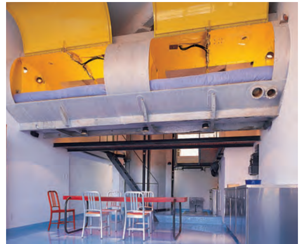
LOT/EK, Morton Residence, New York, 1999. A used petroleum trailer tank was hoisted into this loft, then cut in two sections, one placed vertically and fitted out as a bathroom with a bright yellow interior. The twin section is converted into a sleeping chamber.
