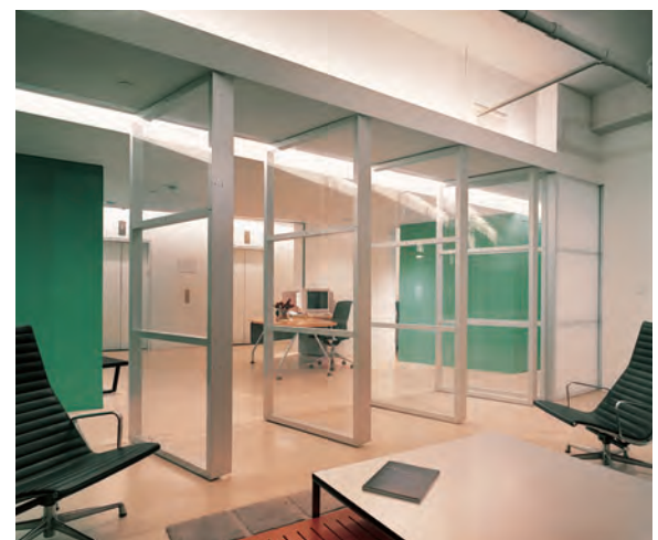
STUDIOS Architecture, RiskMetrics Group, New York, 1999. Translucent and clear acrylic wall panels in a precise grid are attached to aluminum frames with round-headed fasteners. A system of aluminum and glass pivoting doors divides the reception with the conference room, the latter being closed off as needed for meetings. The substantial daylight that filters through the translucent panels is augmented by recessed fluorescent lighting.
