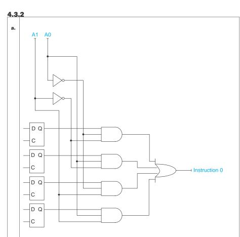
This shows the lowermost bit of each word. This schematic is repeated 7 more times for the remaining seven bits. Note that there are no connections for D and C flip-flop inputs because datapath figures do not specify how instruction memory is written.
