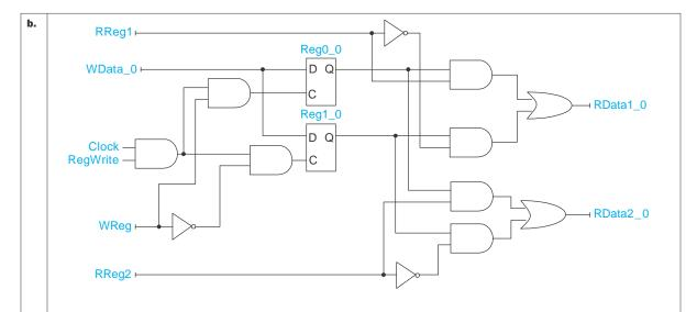
This is the schematic for the lowermost bit, it needs to be repeated 7 more times for the remaining bits. RReg1 is the Read Register 1 input, RReg2 is the Read Register 2 input, WReg is the Write Register input, WData is the Write Data input. RData1 and RData2 are Read Data 1 and Read Data 2 outputs. Data outputs and input have "\_0" to denote that this is only bit 0 of the 8-bit signal.
