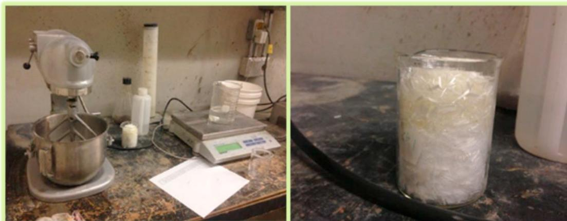
Fig. 3. Measuring and mixing equipment (left); Mixture of PVA and PET fibres (right).
