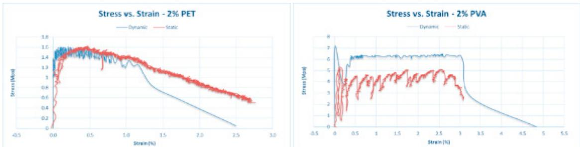
Fig. 9. Stress vs. Strain responses for the 2% PET mix (left) and the 2% PVA mix (right).
