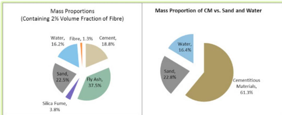
Fig. 2. Mass proportions (left); Mass proportions of CM vs. water and sand (right).
