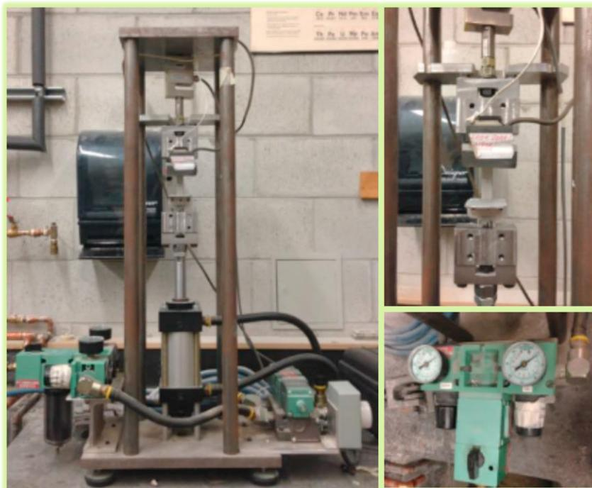
Fig. 5. Dynamic tensile loading apparatus (left), grip mechanism (top right), and the air pressure chamber (bottom right).
