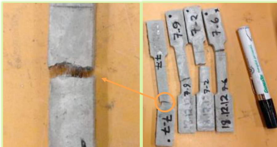
Fig. 6. Tested specimens (right) and the fibre pull out at the crack opening (left).
