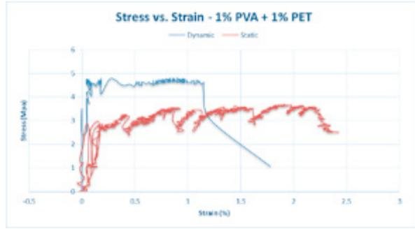
Fig. 10. Stress vs. Strain response for the hybrid mix of 1% PET + 1% PVA.
