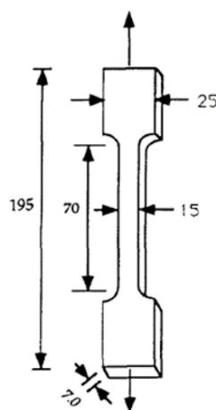
Fig. 1. Sample's dimensions (mm).
