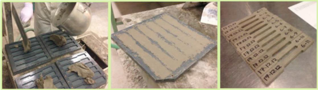
Fig. 4. Casting, moulding, consolidation, and demoulded EDCC Specimens (from left to right).
