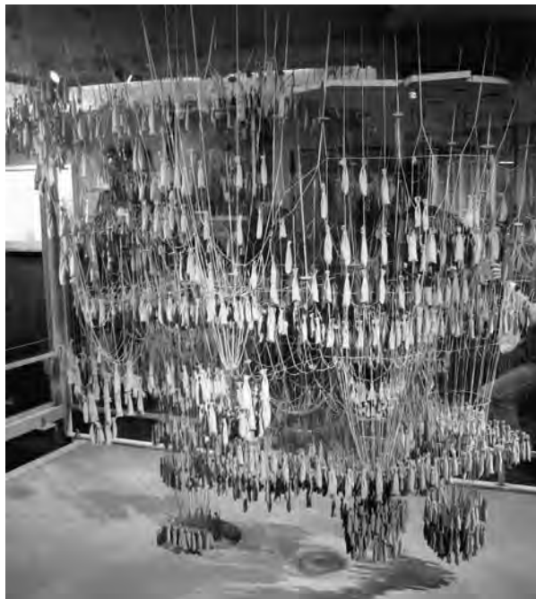
Figure 6.54. One of Gaudí's models of a configuration of strings under loads. Photo by Cleftref
