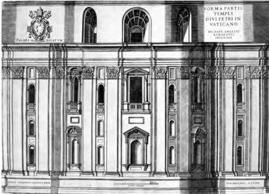
Figure 5.34. Michelangelo's design of the exterior wall of the southern hemicycle of St. Peter's with papal seal of approval, engraving published by Vincenzo Luchino, 1564. From Henry A. Millon and Craig Hugh Smyth, "Michelangelo and St. Peter's I: Notes on a Plan of the Attic as Originally Built on the South Hemicycle," Burlington Magazine , vol. 111, no. 797 (Aug. 1769)
