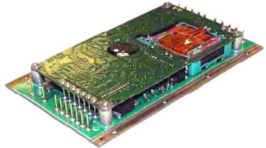
Figure 221 Example of Sub-modular Design
