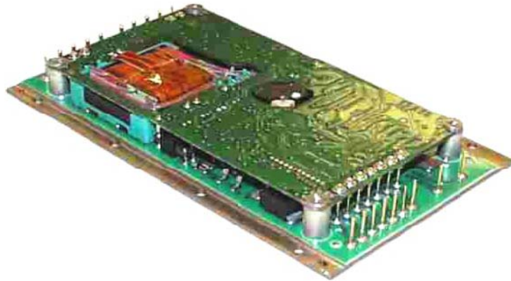
Figure 225 Typical Modular Circuit
