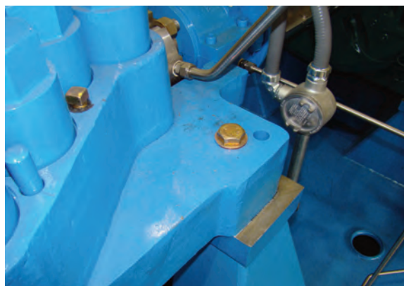
Figure 7. Overhang of Base Pad.
