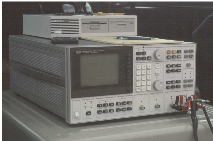
Figure 5-30. Spectrum Analyzer and Data Logging Equipment for SASW.
