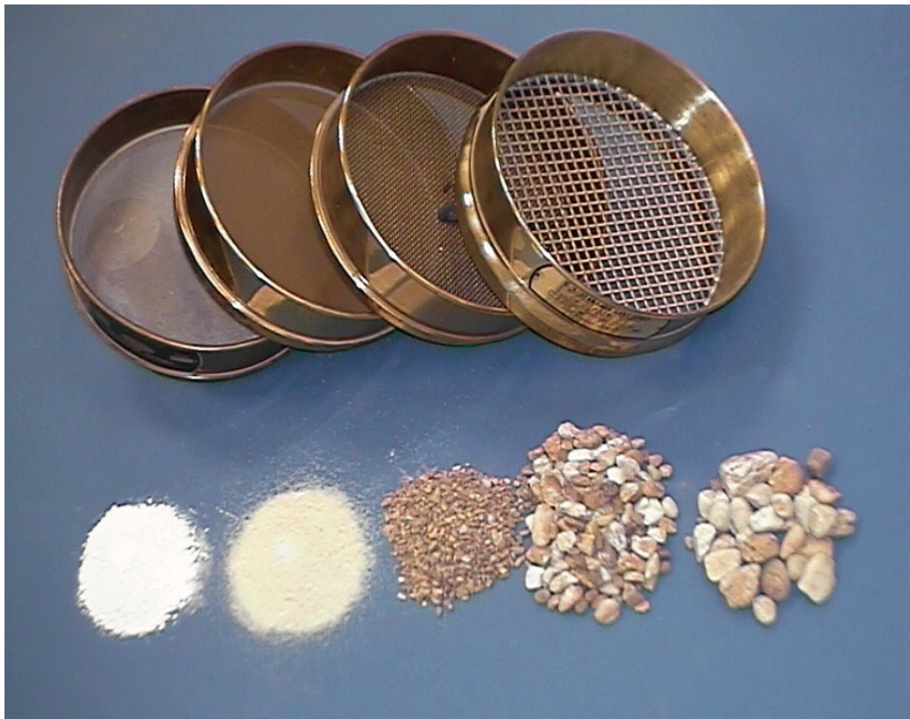
Figure 7-1. Laboratory Sieves for Mechanical Analysis for Grain Size Distributions.
