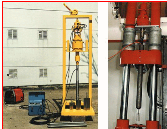
Figure 5-11. Selection of Vane Shear Blades, Pushing Frames, and Torquemeter Devices.
