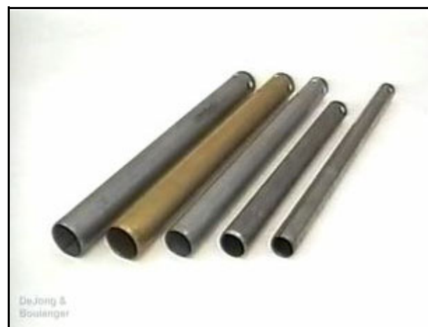
Figure 3-11. Selected Sizes and Types of Thin-Walled Shelby Tubes.
