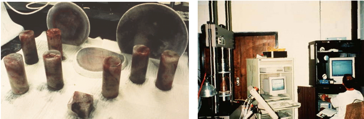
Figure 8-1: (a) Intact Rock Specimens for Laboratory Testing; (b) Compressive Strength Testing.
