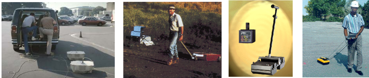
Figure 5-32. Ground Penetrating Radar (GPR) Equipment from Xadar, GeoVision, and EKKO Sensors & Software.
