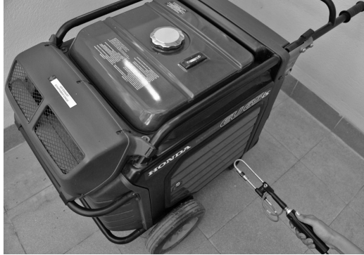
FIGURE 8.5 Sound intensity measurements on a portable generator.
