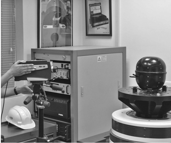
FIGURE 6.8 Compressor vibration measurements using a laser vibrometer.
