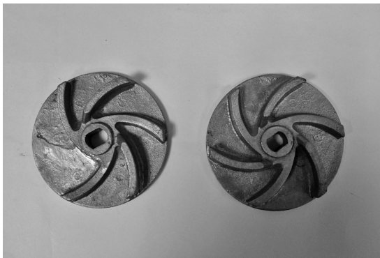
FIGURE 9.7 Broken and normal impeller of submersible pump.
