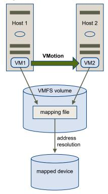
Figure 19-2. vMotion of a Virtual Machine Using Raw Device Mapping
