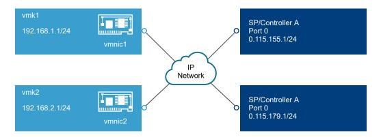
You configure vmk1 and vmk2 in separate subnets, 192.168.1.0 and 192.168.2.0. Your target portals are also in separate subnets, 10.115.155.0 and 10.155.179.0.
