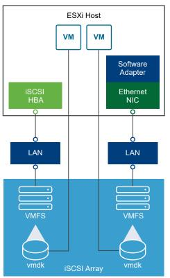
In the left example, the host uses the hardware iSCSI adapter to connect to the iSCSI storage system.
