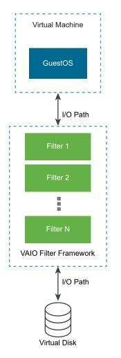
Each Virtual Machine Executable (VMX) component of a virtual machine contains a Filter Framework that manages the I/O filter plug-ins attached to the virtual disk. The Filter Framework invokes filters when the I/O requests move between the guest operating system and the virtual disk. Also, the filter intercepts any I/O access towards the virtual disk that happens outside of a running VM.
