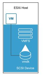
In this example of a local storage topology, the ESXi host uses a single connection to a storage device. On that device, you can create a VMFS datastore, which you use to store virtual machine disk files.
