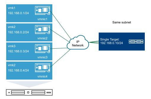
In this example, all initiator ports and the target portal are configured in the same subnet. The target is reachable through all bound ports. You have four VMkernel ports and one target portal, so total of four paths are created.
