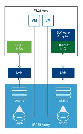
The iSCSI SAN uses a client-server architecture.
