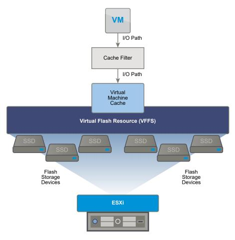
To set up a virtual flash resource, you use flash devices that are connected to your host. To increase the capacity of your virtual flash resource, you can add more flash drives. An individual flash drive must be exclusively allocated to a virtual flash resource and cannot be shared with any other vSphere service, such as vSAN or VMFS.
