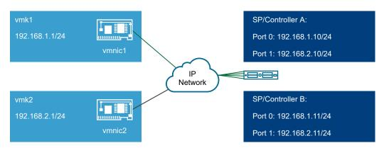
ESXi selects vmk1 when connecting to Port 0 of Controller A and Controller B because all three ports are on the same subnet. Similarly, vmk2 is selected when connecting to Port 1of Controller A and B. You can use NIC teaming in this configuration.
