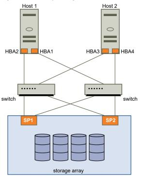
Figure 18-1. Multipathing and Failover with Fibre Channel
