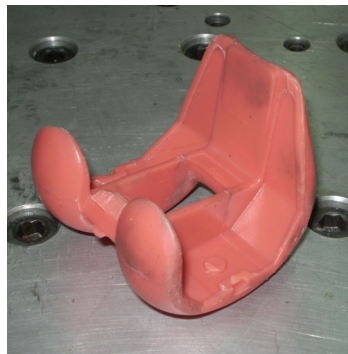
Fig. 7 Meltable wax pattern of knee implant
