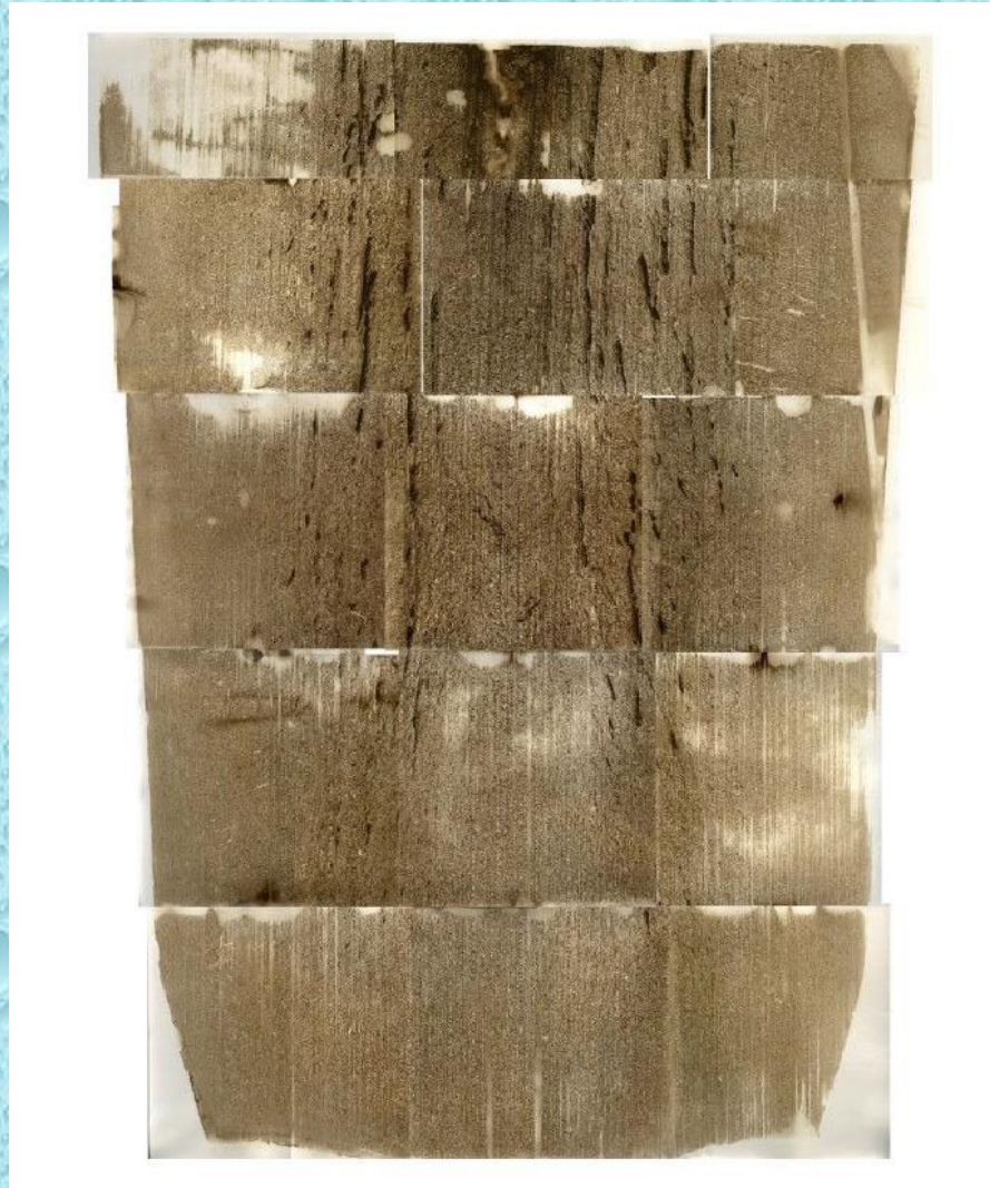
Sulphur print of vertical cross-section of rectangular ingot
