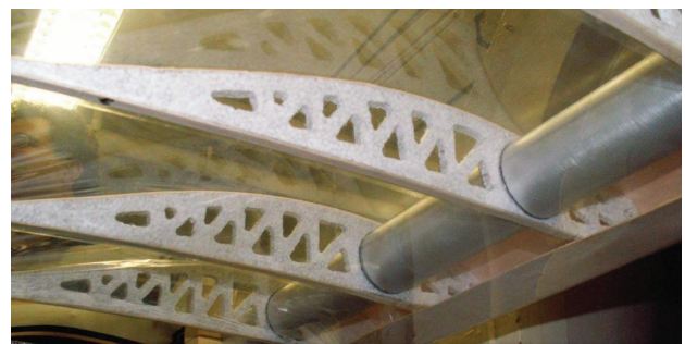
Fig 9. Aluminum Tube Spar
