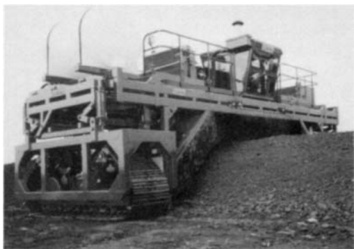
Figure 9-14 Windrow composting machine (courtesy of Scarab Manufacturing).
