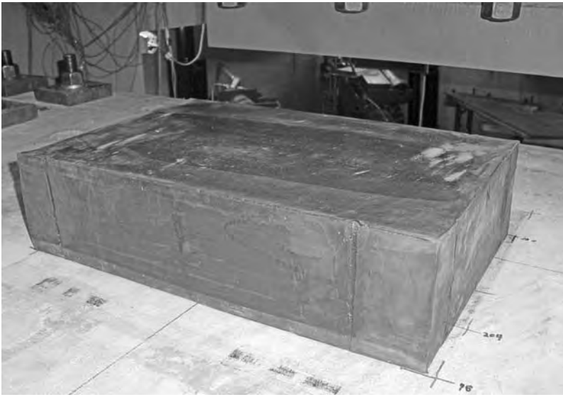
Figure 9.4 A 120-mm-tall unbonded multilayer rubber bearing (plan dimensions: 375 × 575 mm).
