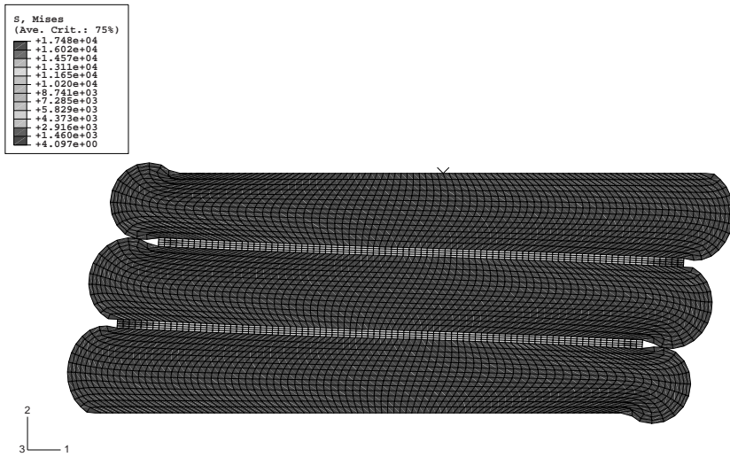
Figure 6.7 Buckled shape and von Mises stresses for Model 5 (compression)
