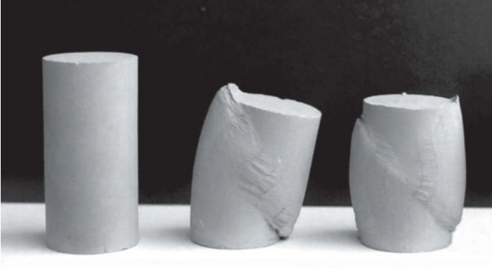
Figure 1.11. Examples of localization of deformation occurring for compressive loads . Shear banding in a 36.5 \times 74.9 -mm cylindrical silty clay sample (the same material used for the tests reported in Fig. 1.5, but now over-consolidated, with over-consolidation ratio equal to 2) subjected to an undrained triaxial compression test. The intact sample before the test is shown on the left. A sample tested with a free top is reported at the centre (in which a single shear band has developed), whereas a fixed top was used for the sample on the right (in which two twin shear bands have developed). Shear bands have emerged before the peak of the stress/strain curve was reached (near 2% axial strain, whereas the test was interrupted at an axial strain near 25%), up to this point, the results of the two tests for the two samples shown at the centre and on the right were near coincident, but the post-peak behaviour was strongly different (softening was more pronounced in the test the with free top; see Fig. 1.18). The qualitative nominal stress versus conventional strain curves corresponding to the samples shown in Figs. 1.5 and 1.11 are reported in Fig. 1.18.
