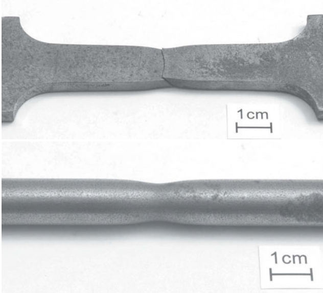
Figure 1.6. Examples of localization of deformation occurring for tensile loads in low-carbon steel samples. Top : Necking is the first mode occurring in the dog-bone-shaped strip shown in the figure. Later, shear banding (with a 45^\circ inclination) develops within the necked zone, which eventually degenerates into a fracture (visible in the photo). Bottom : Necking in a cylindrical bar under tension.
