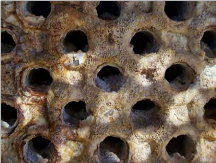
Microbial contamination on a tube sheet
