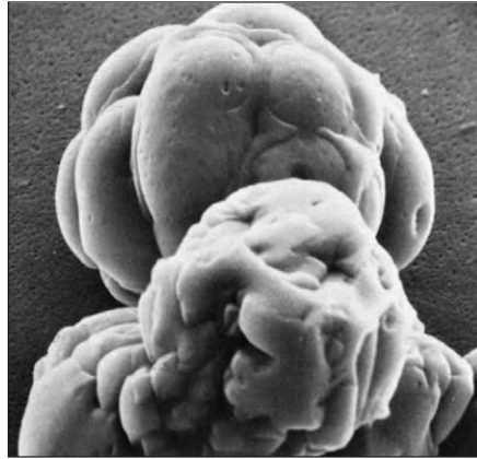
Treatment with a polyacrylate yields distorted calcium carbonate crystals that grow very slowly (magnified 2000X)
