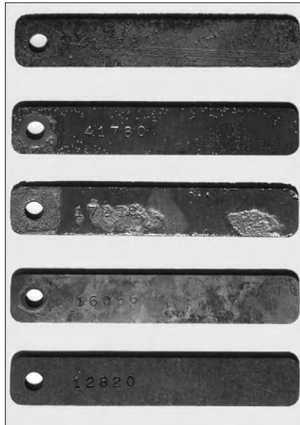
Corrosion coupons inserted into the cooling system can provide an accurate indication of corrosion rates.
