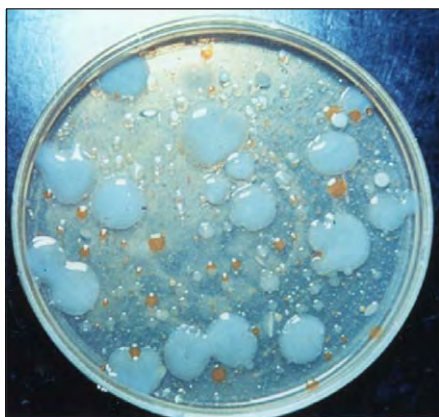
Example of bacterial cultures from cooling water system grown on an agar plate as part of a DMA
