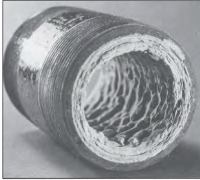
Calcium carbonate scale
