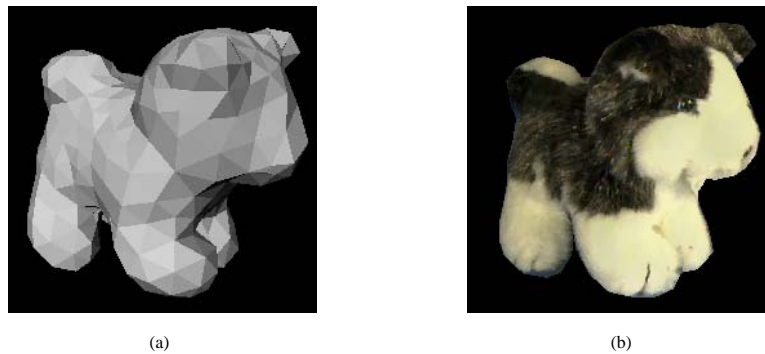
Figure 15.16: Rough mesh model of a dog and texture-mapped image. Courtesy of Kari Pulli.
