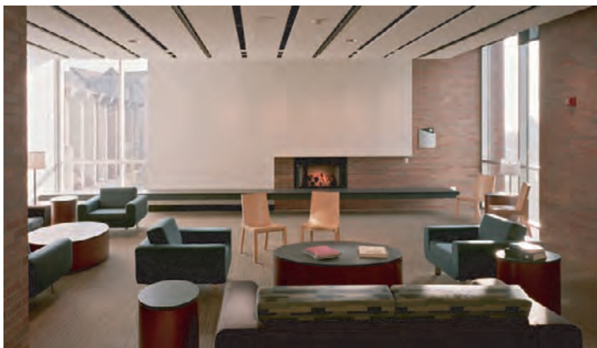
4.81 A lounge in the Christopher Center at Valparaiso University, Indiana, demonstrates a "wall washing" daylighting technique with the glazing aperture directly adjacent to a light-colored wall. © PETER AARON/ESTO
