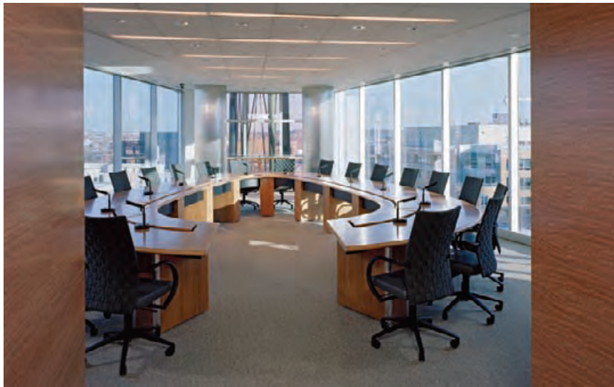
5.98 Expansive views from a conference room which has carpet tiles with recycled content and low VOC. Ceilings are of mineral fiber acoustical tiles with more than 65% recycled material. © ALAN KARCHMER
