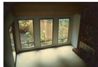
4.57 Scale models (such as of the residence shown above) can be used to predict daylight factor during design. Surface reflectances must be carefully modeled for accurate predictions.
