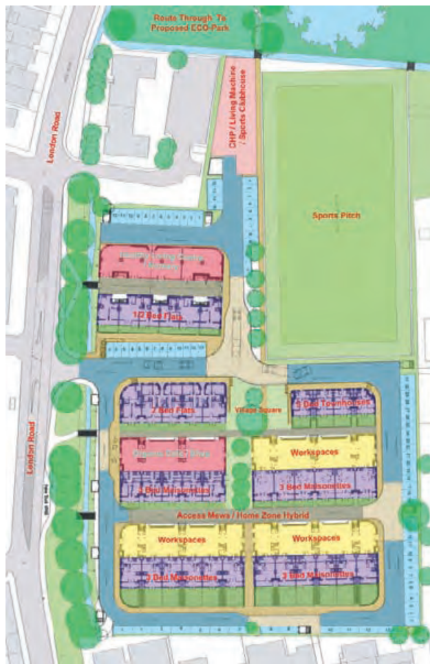
5.16 BedZED site plan. Residential (purple) is on the south side of each terrace, with workspaces (yellow and orange) to the north. BILL DUNSTER ARCHITECTS/ZEDFACTORY.COM
