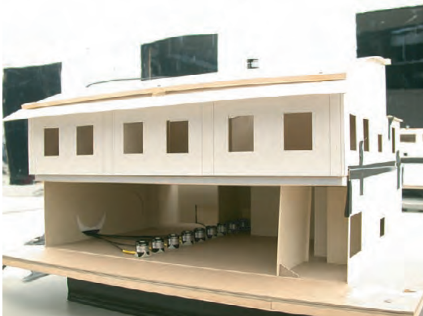
4.59 Daylight model placed in an artificial sky with several interior photosensors and a single exterior sensor (on roof) to measure illuminances and determine daylight factors. The model is “unglazed” and the additional daylight this admits will be corrected for when calculating DF.
