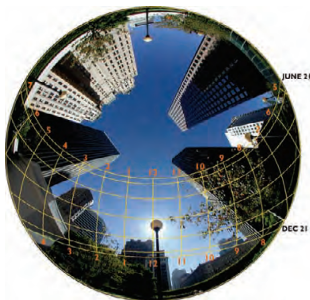
4.103 Sun path chart overlain onto a fisheye photo of the sky. ROBERT MARCIAL
