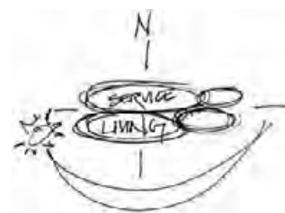
4.123 Unoccupied or service spaces can be placed along the cooler non-solar facade, leaving the warmer side for living spaces.
