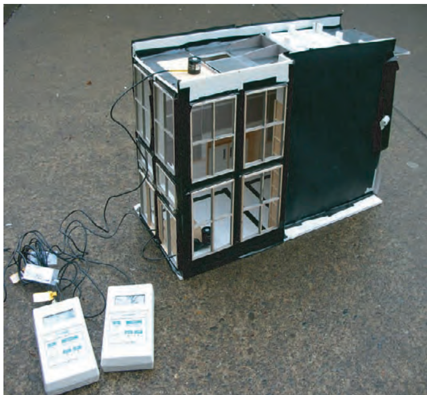
4.60 Daylight model being tested outdoors under an overcast sky with an interior and exterior photosensor to measure illuminances and calculate daylight factor.
