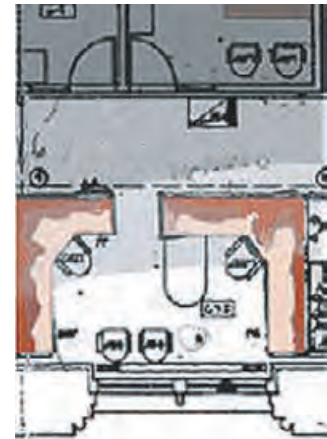
4.61 Isolux plot of measured daylight zones in an office building.
