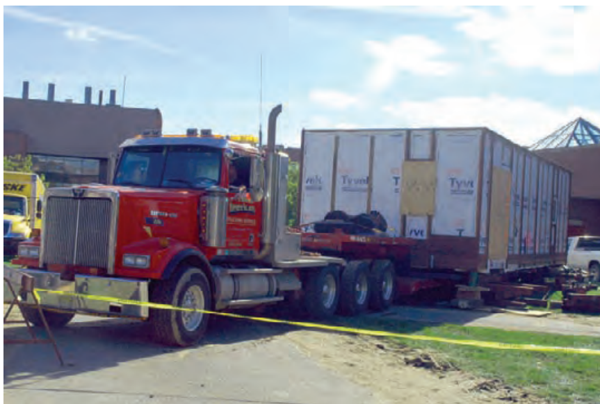
5.35 Shipping constraints drove much of the design and the ultimate form of the Cornell House. NICHOLAS RAJKOVICH
