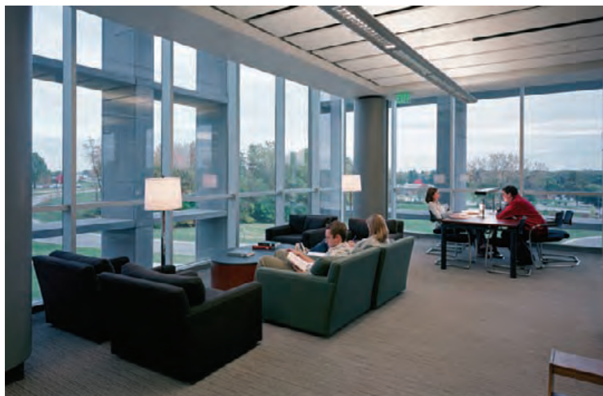
4.119 Integrated electric lighting and daylighting in a reading area of the Christopher Center at Valparaiso University, Indiana. © PETER AARON/ESTO
