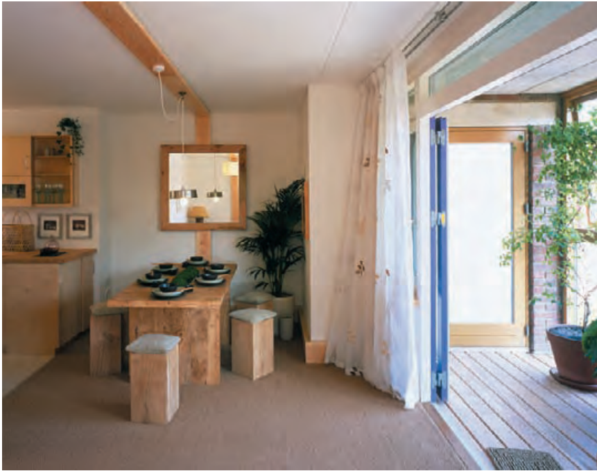
5.22 Sunspaces in the residential units provide solar gain and extended living space when the weather allows. GRAHAMGAUNT.COM
