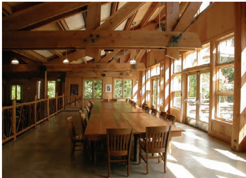
4.124 Concrete floors absorb solar radiation in the direct gain dining hall of IslandWood Campus on Bainbridge Island, Washington.
