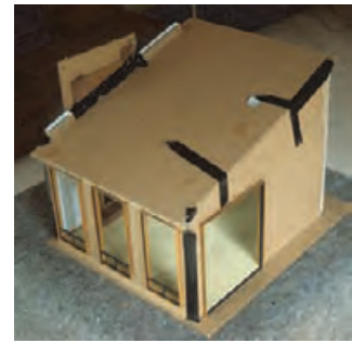
4.53 Exterior view of a typical daylighting study model.
