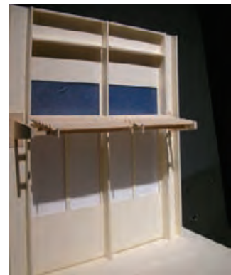
4.105 Performance of proposed shading device at 3:00 p.m. on June 21.
