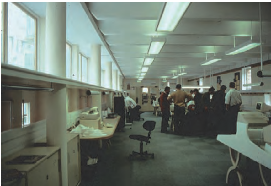
4.65 Daylit computer area in the Queen's Building at DeMontfort University in Leicester, UK, showing coordination of electric lighting fixtures with sidelighting zones. THERESE PEFFER
