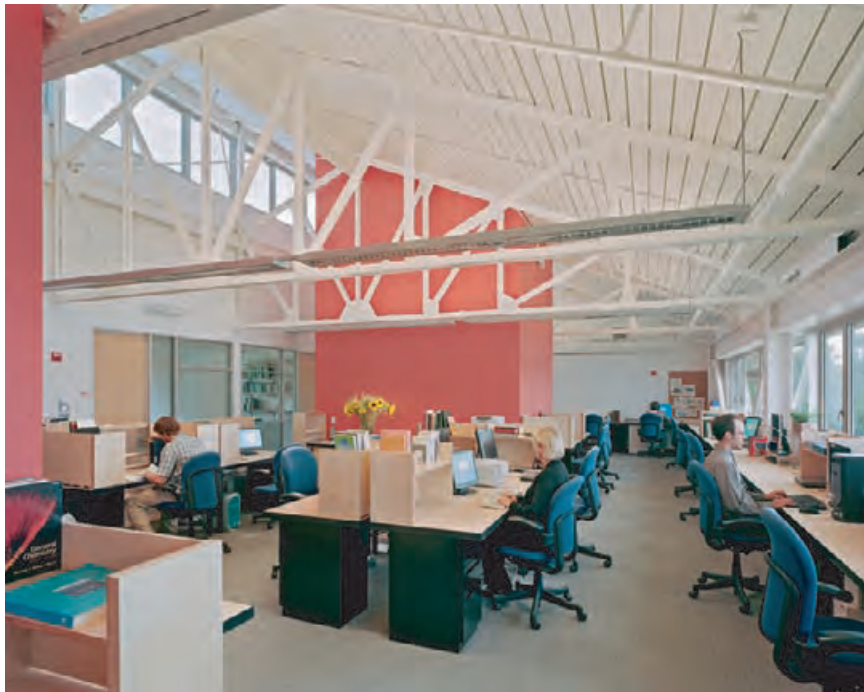
4.80 Bilateral sidelighting from view windows and clerestories in a computer lab at the Global Ecology Research Center at Stanford University, Palo Alto, California. © PETER AARON/ESTO
