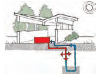
4.143 Ground source heat pump using a vertical ground loop. KATE BECKLEY
