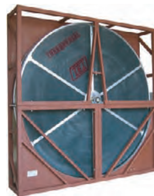
4.212 An industrial grade energy recovery wheel designed to handle airflow volumes from 15,000 to 150,000 cfm [7080 to 70,785 L/s] with a total effectiveness of up to 90%. Wheel diameters range from 6 to 20 ft [1.8–6.1 m]. THERMOTECH ENTERPRISES, INC.
