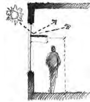
4.84 Conceptual sketch of a light shelf in an office. GREG HARTMAN
