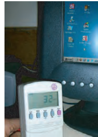
4.203 Watt meter showing a desktop computer monitor using 32 watts when in active mode.
