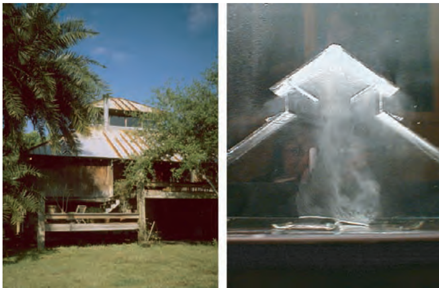
4.162 The Logan House (left), Tampa, Florida, a well-studied example of stack effect ventilation. Bubble-testing a model of the Logan House (right) to determine stack performance and examine alternative window configurations. ALISON KWOK | CHRISTINA BOLLO
