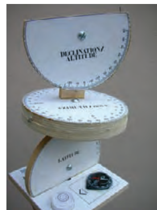
4.101 The solar transit is a useful device to trace the sun's path across the sky and create horizon shading masks for a particular location.
