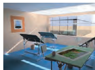
4.58 A computer simulation, such as Radiance, can provide daylight factor predictions and facilitate qualitative evaluation of a proposed design. GREG WARD
