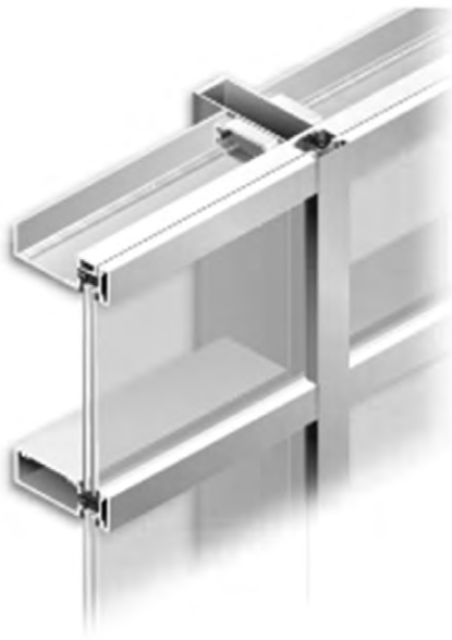
Fig. 3-12. Tubular mullion system
