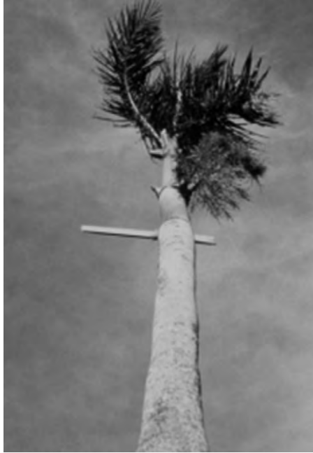
Fig. 4-9. Close-up of the projectile embedded in a palm tree Source: http://www.photolib.noaa.gov/brs/nwind12.htm ; courtesy of NOAA
