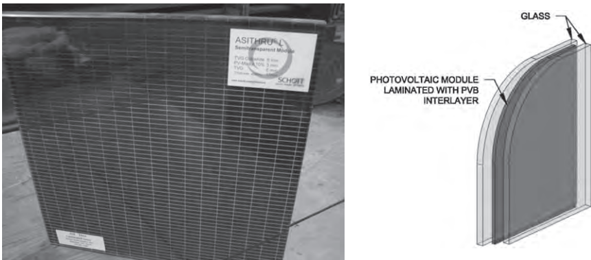
Fig. 11-6. Photo showing sample of laminated glass with crystalline cells within the laminate and a drawing showing the layers
