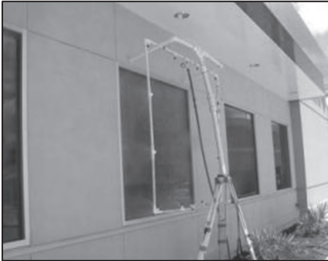
Fig. 4-16. A spray rack test AAMA 503
