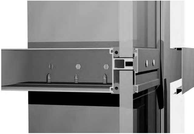
Fig. 7-8. A pressure plate connects a panel surface to a horizontal beam; a shear plate connects a horizontal beam to a vertical mullion
