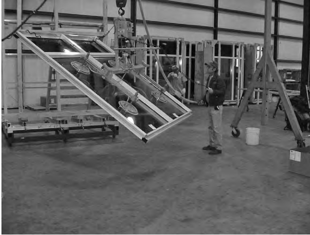
Fig. 3-16. Unitized or shop-assembled system
