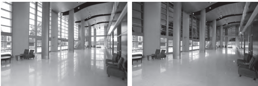
Fig. 10-15. Nonactivated (left) versus activated (right) electro-chromic glass (Sage Electronics 2013)
