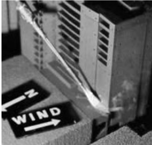
Fig. 4-20. Representative wind dispersion study using smoke
