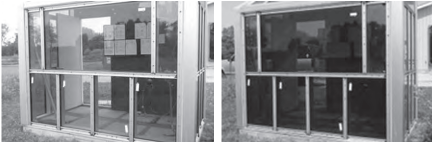
Fig. 10-14. Nonactivated (left) versus activated (right) thermo-chromic glass (Plotint 2013)
