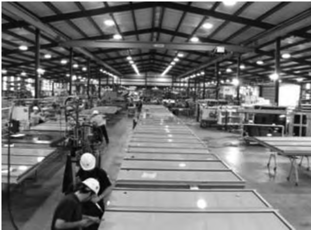
Fig. 3-15. Unitized or shop-assembled system
