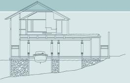
through the holes to settle on the lakebed. Before the holes in the ice freeze over, granite rocks are dropped into the cribs as ballast."
