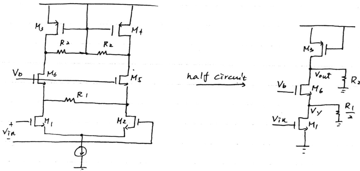
$$\frac{V_y}{V_{in}} = -g_m \left( \frac{1}{g_m R_1} // \frac{R_1}{2} \right), \quad \frac{V_{out}}{V_y} \approx +g_m \cdot R_2$$
