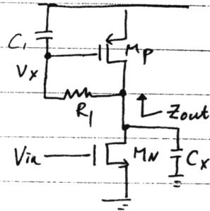
(i) At low frequency,  $C_1$  is open circuit. $M_p$  is like a diode-connected device  $\rightarrow Z_{out} \sim \frac{1}{g_{mp}}$ (ii) At high frequency,  $C_1$  is short circuit. $M_p$  is like a current source device  $\rightarrow Z_{out} \sim (r_{on} // r_{op})$ Since  $(r_{on} // r_{op}) \gg \frac{1}{g_{mp}}$ ,  $Z_{out}$  exhibits an inductive behavior
