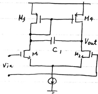
$C_1$  is like an open circuit @ very low frequency
