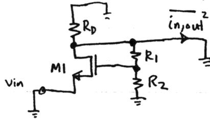
$$\begin{aligned} \overline{i_{n,out}^2} &= 4kT \frac{1}{R_D} + 4kT \frac{2}{3} g_{m_1} + \overline{i_{noise,R_1}^2} + \overline{i_{noise,R_2}^2} \\ \overline{i_{noise,R_1}^2} &= 4kT \frac{1}{R_1} |A_{I,R_1}|^2 \\ \overline{i_{noise,R_2}^2} &= 4kT \frac{1}{R_2} |A_{I,R_2}|^2 \end{aligned}$$
