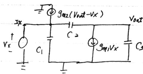
$$I_x = SC_1V_x + SC_2(V_x - V_{out}) + g_{m2}(V_x - V_{out})$$
