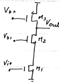
The impedance @  $V_{out}$  =  $\frac{1}{g_{m3}}$
