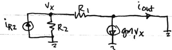
$$A_{I,R_2} = \frac{i_{out}}{i_{R_2}} = \left[ \frac{R_2}{R_1 + R_2} - gm_1 (R_1 // R_2) \right]$$
