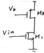
$$Av = -g_{m1} (r_{o1}/r_{o3}) \rightarrow 0 \text{ if } \lambda = 0$$
