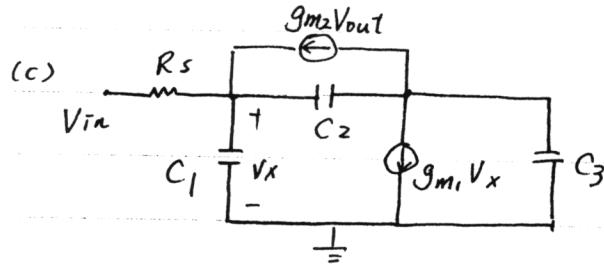
$$\begin{aligned}C_1 &= C_{gs1} + C_{db2} + C_{gd2} \\C_2 &= C_{gd1} \\C_3 &= C_{db1} + C_{sb2} + C_{gs2}\end{aligned}$$
