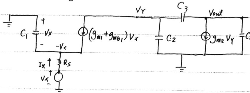
$$C_1 = C_{gs1} + C_{SB1}$$
