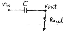
Thus, when there is a step  $\Delta V$  at the input, output will follow input, a step  $\Delta V$ , first.Then, it will settle down to  $-AV_{in}$  as the steady state(b) KCL @  $V_{out}$ :
