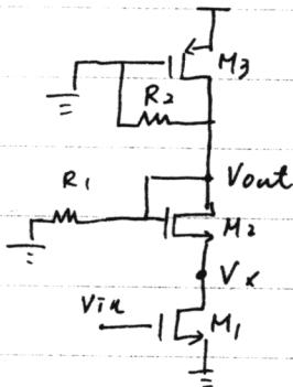
$$\frac{V_X}{V_{in}} = -g_{m1} \cdot \frac{1}{g_{m2}}$$
