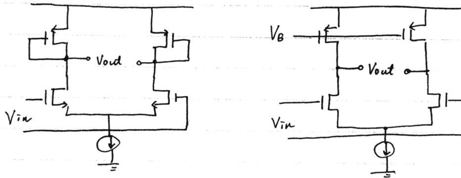
Both of these two differential pair can be simplified as common-source amplifier with different load resistance and capacitance
