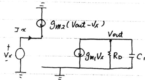
$$V_{\text{out}} = -g_{m1}V_x \left( R_D \parallel \frac{1}{SC_1} \right)$$
