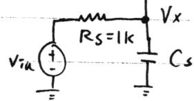
$$\frac{V_{out}(s)}{V_{in}(s)} = \frac{(g_m + g_{mb}) R_D}{1 + (g_m + g_{mb}) R_s} \cdot \frac{1}{\left(1 + \frac{C_s}{g_m + g_{mb} + R_s^{-1}} \cdot s\right) (1 + R_D C_D s)}$$
