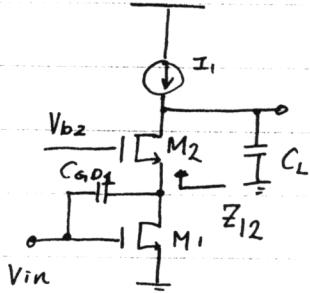
The impedance  $Z_{12}$  can be derived from the following small signal model
