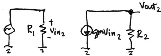
$$Av_2 = \frac{V_{out2}}{Vin_2} = -gm R_2 = \frac{-gm R_F Av_1}{Av_1 - 1} = (-gm R_F + 1) = Av_1$$
