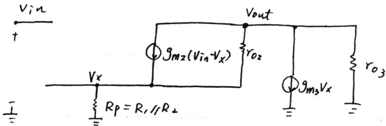
$$KCL @ V_x, V_{out} : \frac{V_x}{R_p} = g_{m2}(V_{in} - V_x) + \frac{V_{out} - V_x}{r_{o2}} = -(g_{m3}V_x + \frac{V_{out}}{r_{o3}})$$
