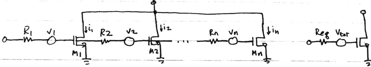
The drain noise current of  $M_1$  resulting from the gate resistance is
