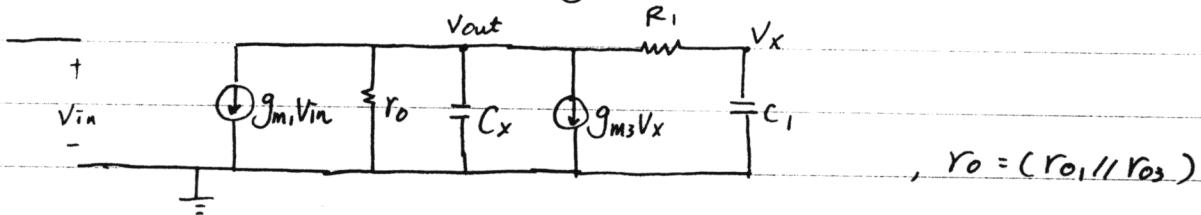
KCL @  $V_x$  :  $\frac{V_{out} - V_x}{R_1} = SC_1 V_x \Rightarrow V_{out} = (1 + s R_1 C_1) V_x$
