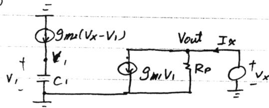
$$\text{KCL at } V_1 : g_{m2}(V_x - V_1) = SC_1 V_1,$$
