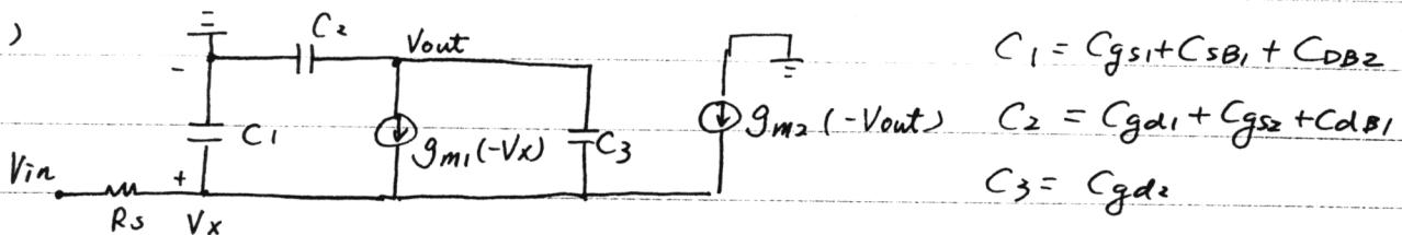
$$C_1 = C_{gs1} + C_{sB1} + C_{dB2}$$
