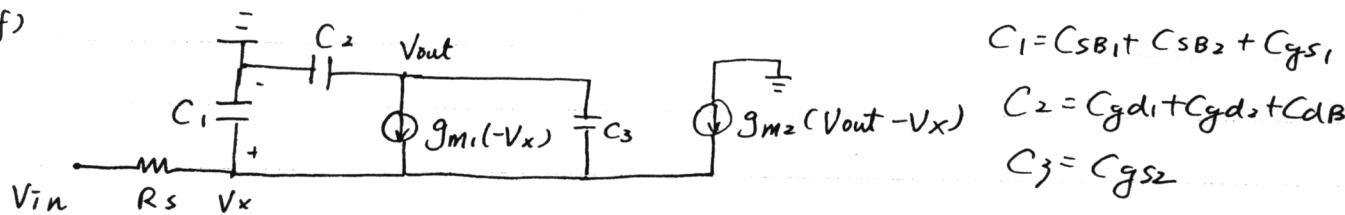
$$C_1 = C_{SB1} + C_{SB2} + C_{gs1},$$
