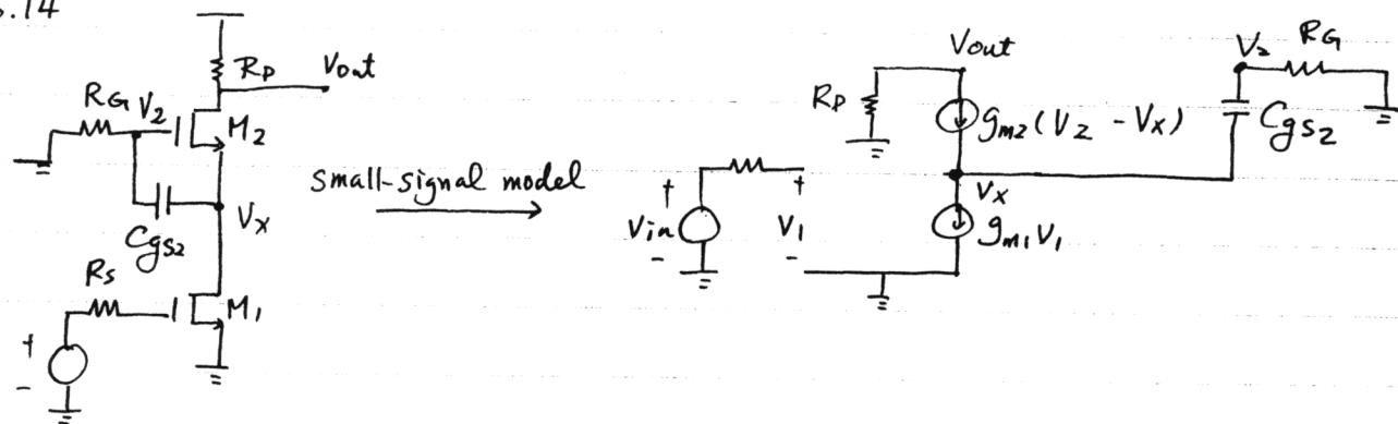
$$\text{KCL at } V_2 : \frac{V_2}{R_g} = sC_{gs2}(V_x - V_2)$$
