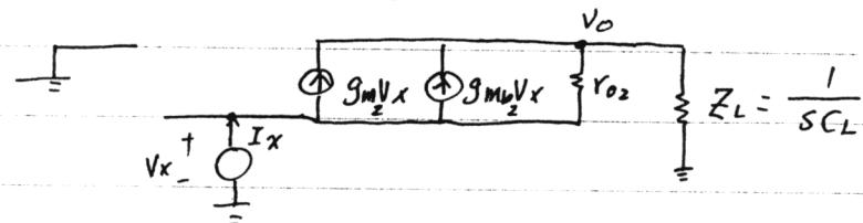
$$\text{KCL at } V_o : \frac{V_o}{Z_L} + \frac{V_o - V_x}{R_{o2}} = (g_{m2} + g_{mb2})V_x \Rightarrow \left( \frac{1}{Z_L} + \frac{1}{R_{o2}} \right) V_o = (g_{m2} + g_{mb2} + \frac{1}{R_{o2}})V_x$$
