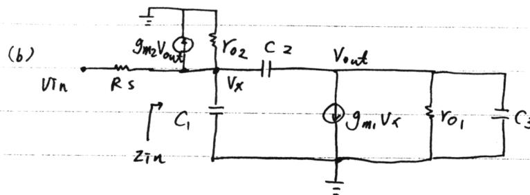
$$C_1 = C_{gs1} + C_{dB2}$$
