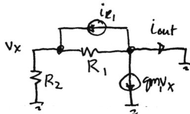
$$A_{I,R_1} = \frac{i_{out}}{i_{R_1}} = -\left( 1 + (R_1 // R_2)(g_{m_1} - \frac{1}{R_1}) \right)$$
