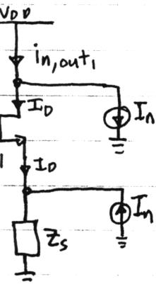
$$I_{n,out} = I_D + I_n, \text{ KCL @ drain}$$
