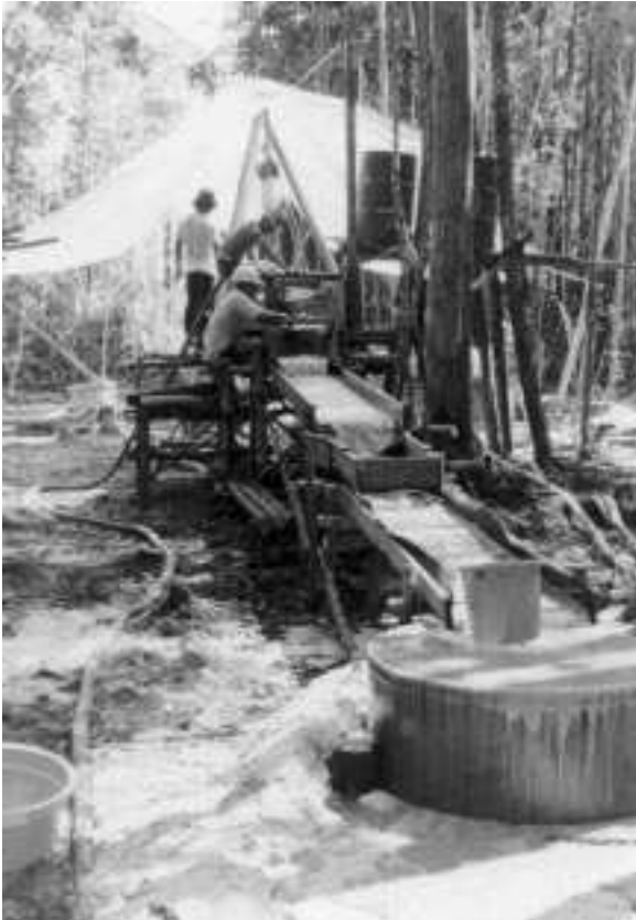
6.31 Long tom sampling arrangement – Ampulit, Kalimantan, Indonesia.
