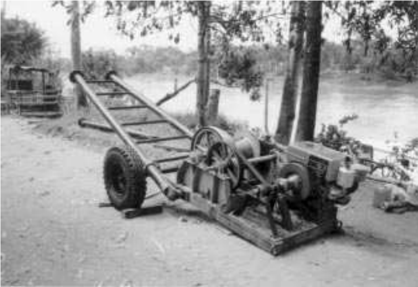
6.10 Sparkes mechanical Banka drill in travelling mode.
