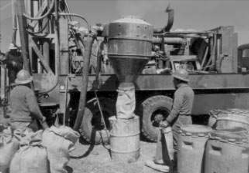
6.18 Sample collecting using cyclone separator – San Antonio de Poto glacial outwash, Peru.
