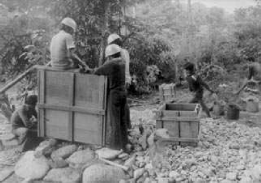
6.7 Pit sample measurement box at dressing site, Krung Cuk, Aceh, Indonesia.
