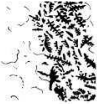
Dentic, flake and plate-like crystal groups of gold (black) in extremely fine-grained quartz of probable colloidal origin. National Mine, Nevada – gold in rhyolite deposit (magnified \times 15 )
