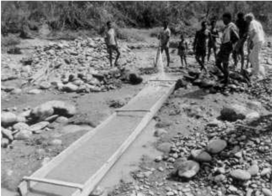
7.8 Ground sluicing a point bar in Lower Waria River, Papua New Guinea.
