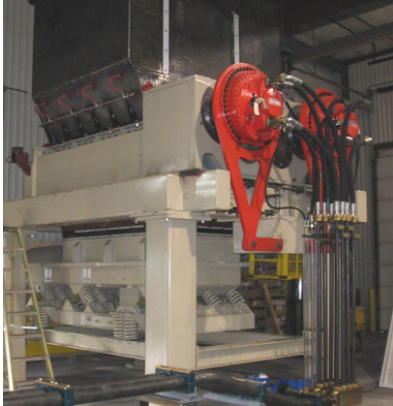
Figure 3: Potential overheating of an industrial shredder is an important consideration in the design of its transmission and bearings.
