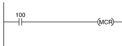
Figure 1.8 Master Control Relay
