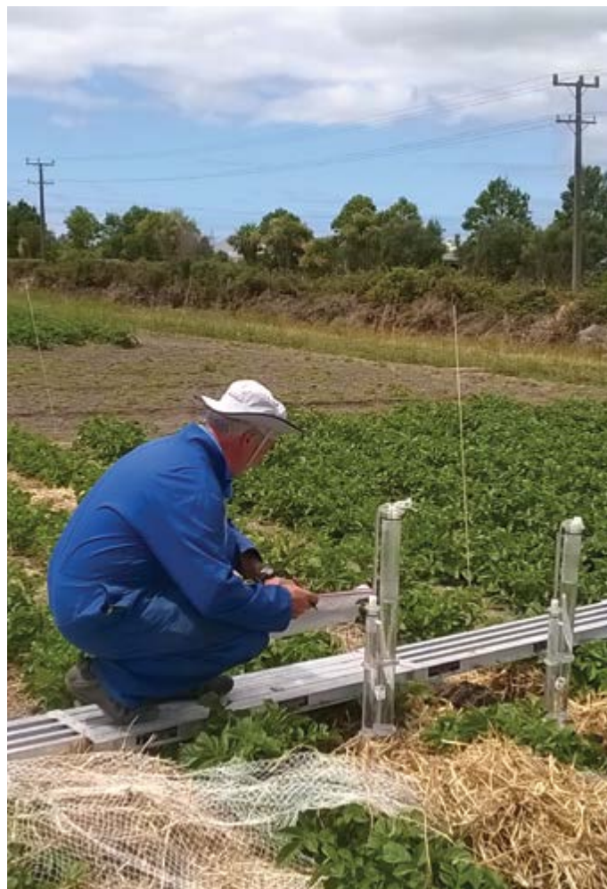
Photo 2: Measuring soil infiltration rates on flat beds.
