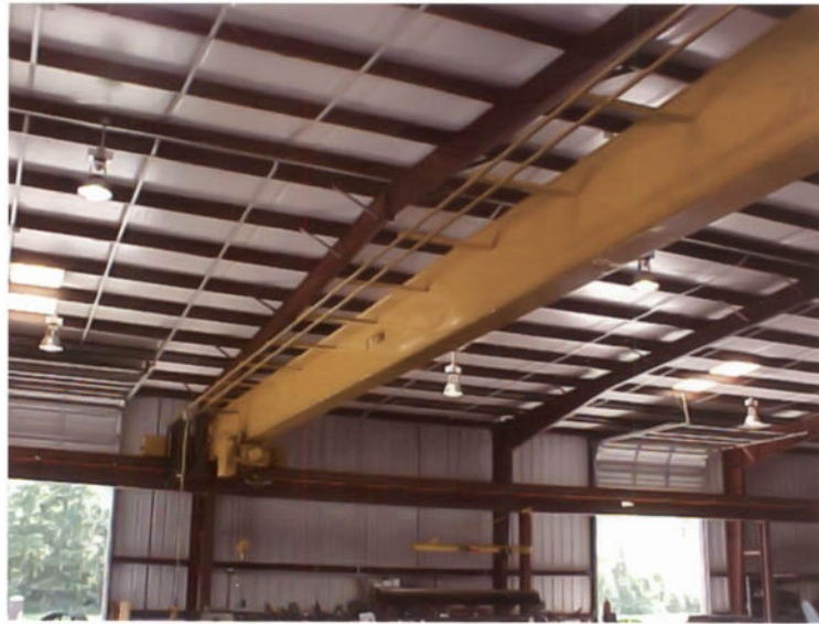
Crane self-supporting for vertical loads but not self-supporting for lateral loads
