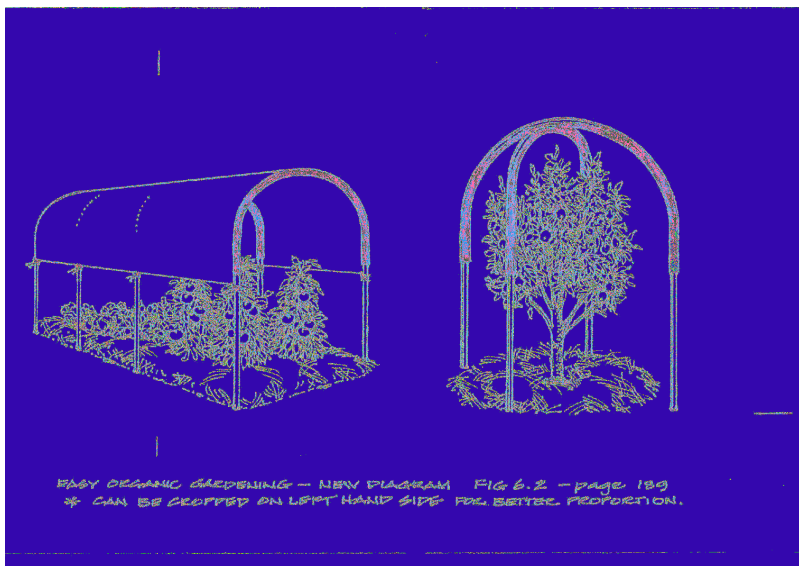
Fig. 6.2 Canopies supported by polypipe arches make it easy to protect precious crops from sunburn, frost, birds and flying foxes..
