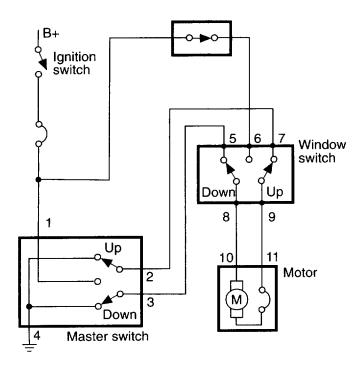
90. The power window motor in the figure shown is completely inoperative. With the master window switch placed in the "down" position, the following voltages are measured at each terminal:
