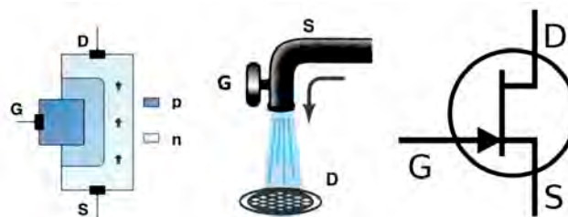
Figure 1. Scheme of an n-channel JFET (left), its hydraulic analogy (middle) and electric circuit symbol (right). The arrows in the JFET scheme indicate the flow of the electric current between Source (S) and Drain (D) through the narrow n-channel. The width of the channel depends on the applied voltage between the Gate (G) and the Source (S).
