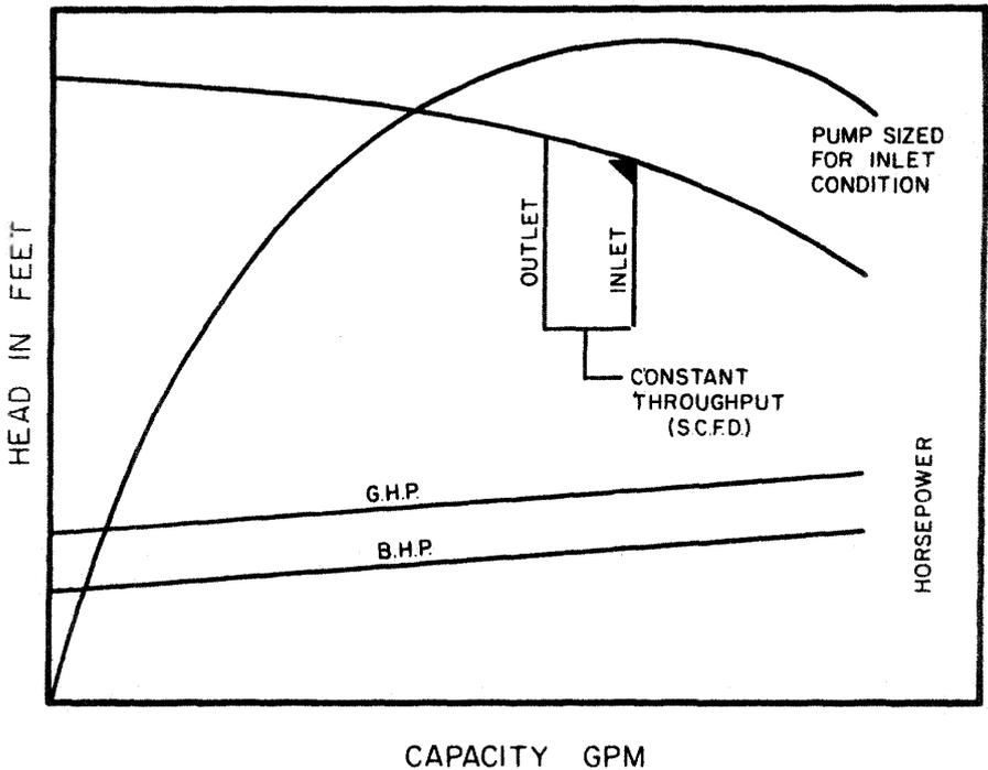
Figure 10-36. Performance curve for CO<sub>2</sub> pump.
