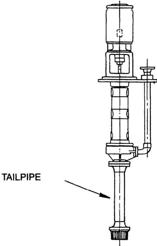
**Figure 15-17.** Vertical sump pump with tail pipe.
