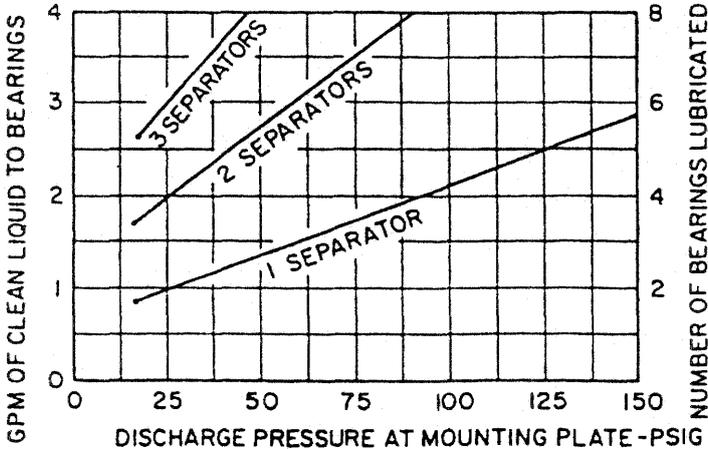
Note: Add 2 gpm per separator to total flow requirements of pump to allow for flow taken by separators.
