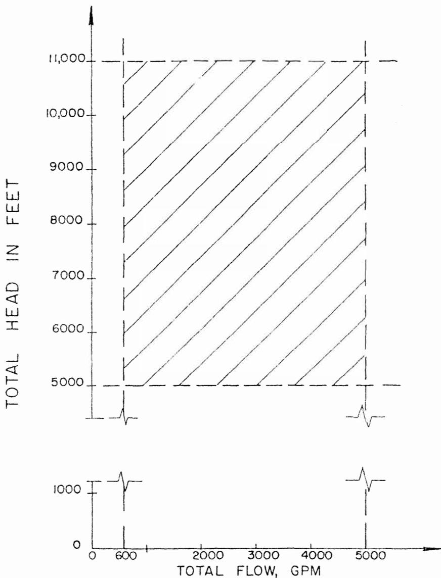
Figure 10-33. Performance coverage for typical waterflood applications.
