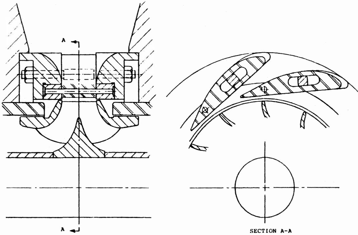
Figure 14-14. Internally adjustable guide vane assembly (courtesy of Bingham- Willamette Company).
