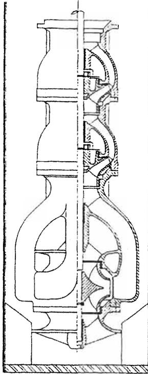
Figure 9-13. Bowl assembly with double suction first stage.
