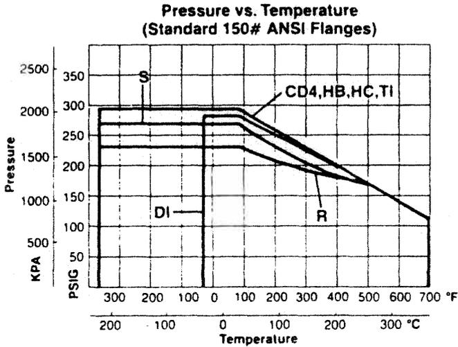
Figure 15-6. Pressure versus temperature for 150 pound ANSI flange.
