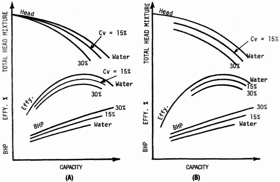
**Figure 13-11.** (A) Typical performance characteristic of nonsettling slurries; (B) typical performance characteristic of settling slurries.
