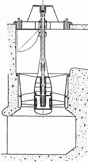
**Figure 9-12.** Propeller pump partly formed in concrete.
