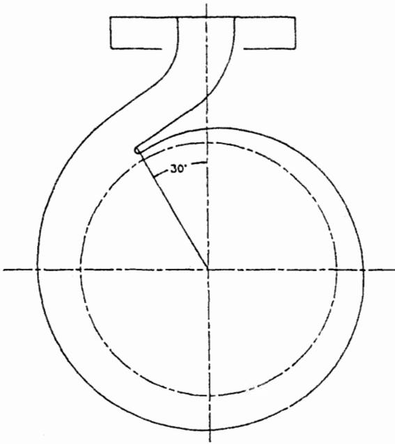
**Figure 15-10A.** Casing volute with centerline discharge nozzle.
