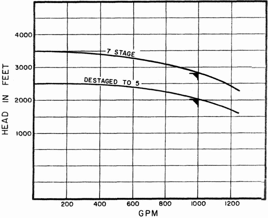
Figure 10-14. Pump performance before and after destaging.
