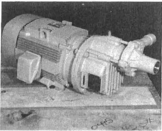
with high-speed pumps can be virtually eliminated without efficiency sacrifice via inducer and staging options. It is interesting to note that a two-stage machine with equal head split optimizes at 60% of single-stage speed, which can reduce NPSHR up to about 70%.
