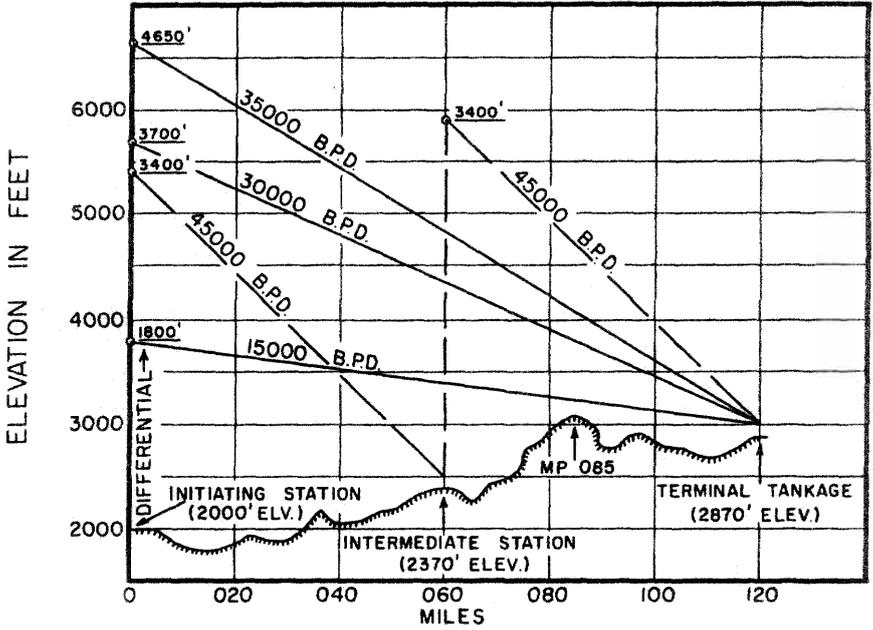
Figure 10-23. Hydraulic gradient and profile of 120-mile-long pipeline.
