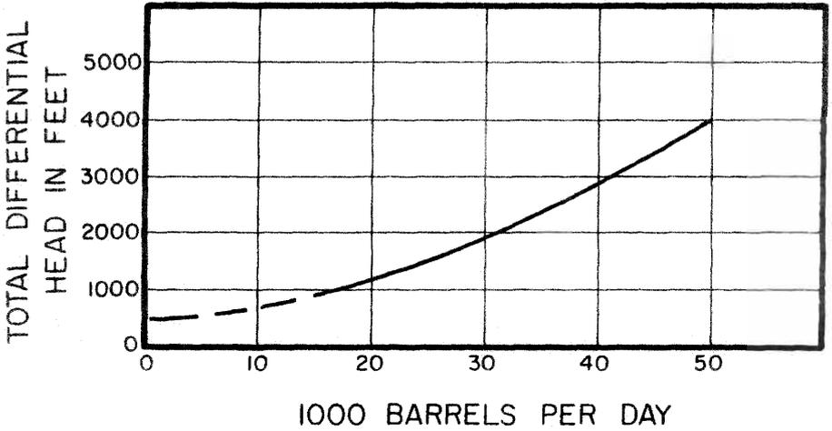
Figure 10-29. System head curve for 45,000 BPD production.
