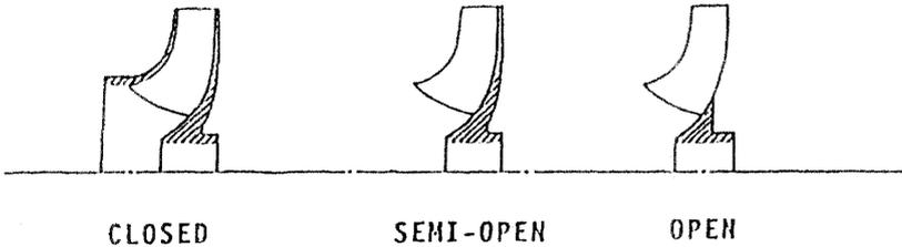
**Figure 9-15.** Impeller configurations.
