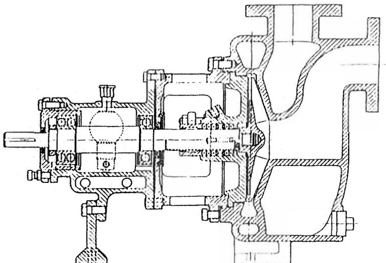
**Figure 15-18.** Self-primer overhung single-stage (courtesy of Goulds Pumps, Inc.).
