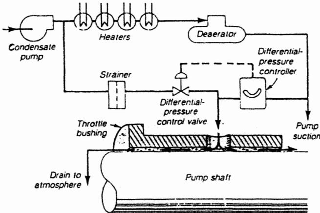
Figure 12-9. Pressure-controlled throttle bushing injection system (from Ashton [2]).
