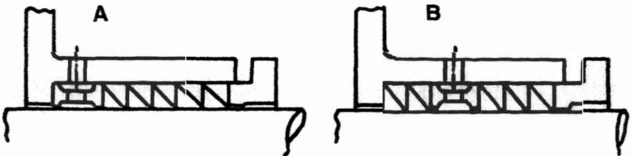
**Figure 13-5.** (A) Typical "flush-type" slurry pump stuffing box. Barrier flush prevents abrasive wear. (B) Typical "weep-type" stuffing box. It uses considerably less gland water but is much more susceptible to abrasive wear.
