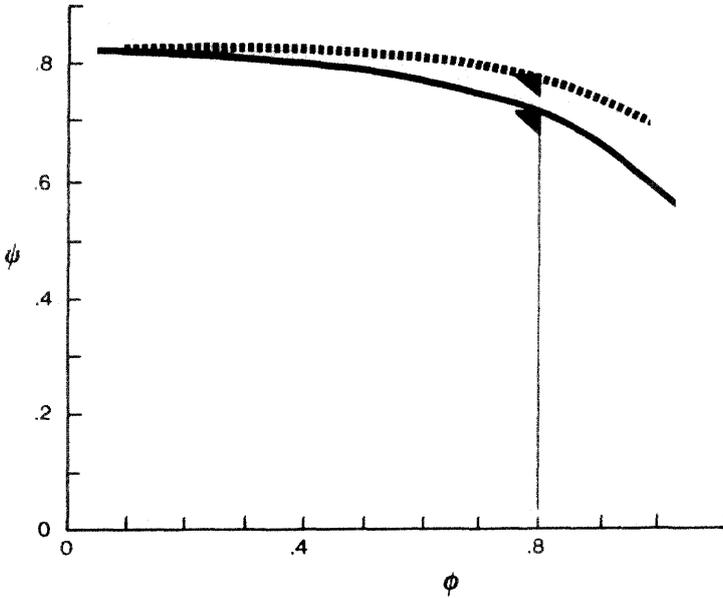
Figure 11-10. Curve shape variation with impeller eye size.
