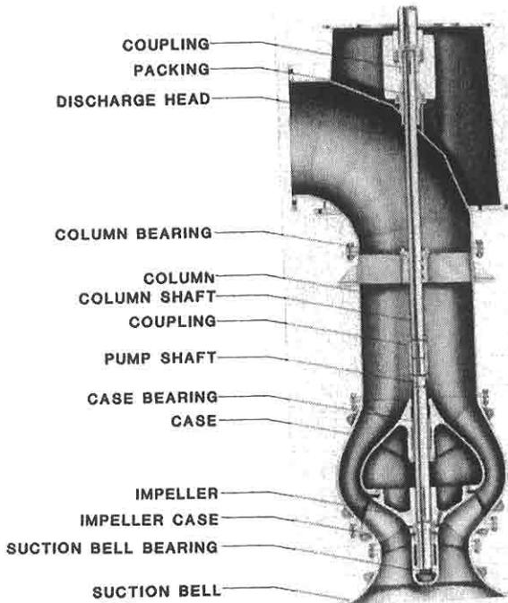
**Figure 9-5.** Wet pit pump (courtesy BW/IP International, Inc. Pump Division, manufacturer of Byron Jackson/United™ Pumps).
