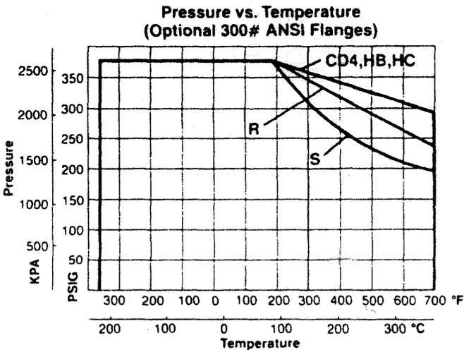
Figure 15-7. Pressure versus temperature for 300 pound ANSI flange.
