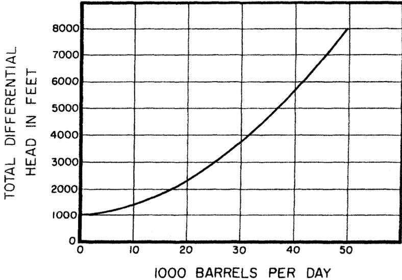
Figure 10-24. System head curve for 15,000 to 30,000 B.P.D. production.
