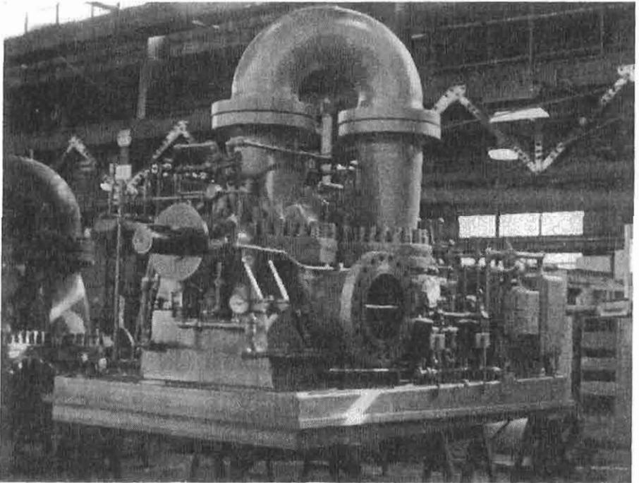
**Figure 10-17.** Two stage pipeline pump with bolted on crossover.
