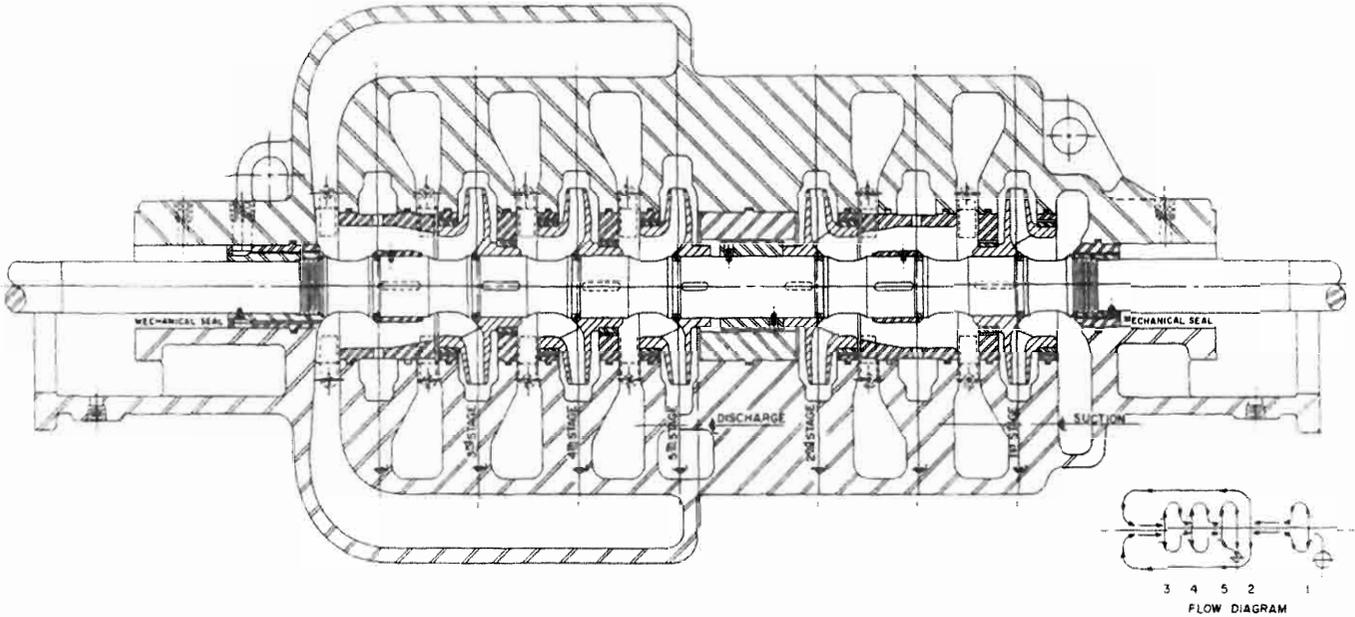
**Figure 10-13.** Seven-stage pump destaged to five stages.
