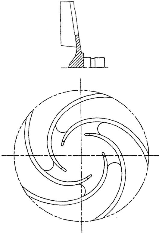
**Figure 15-9A.** Fully scalloped open impeller.
