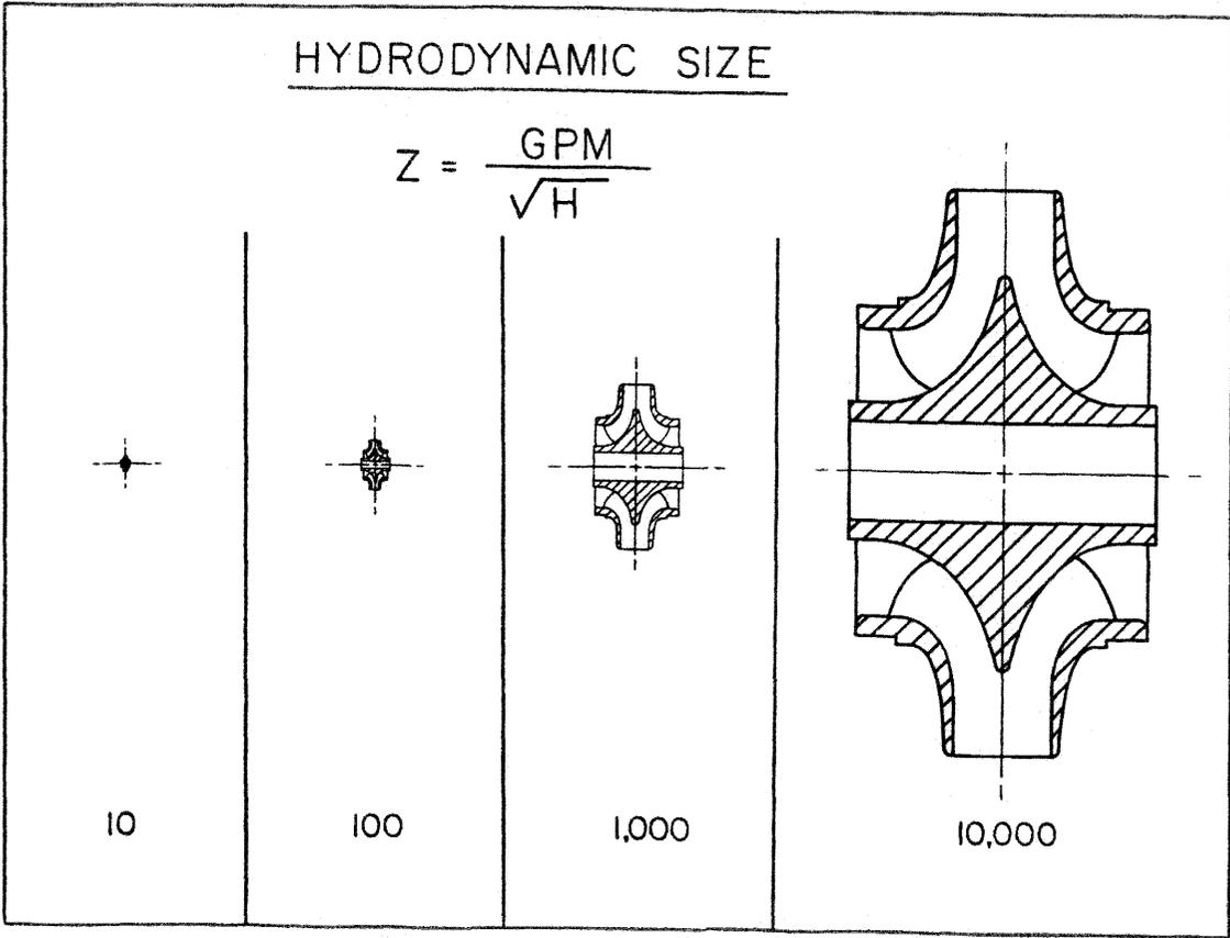
Figure 10-3. Pump size increases with hydrodynamic size.
