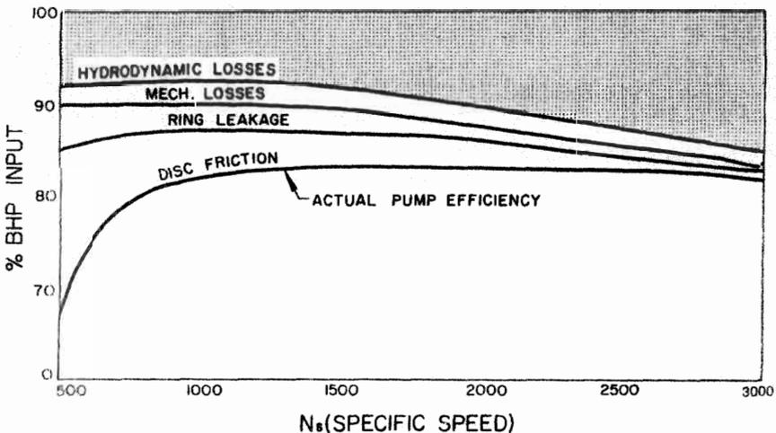
Figure 10-1. Typical analysis of pump losses.
