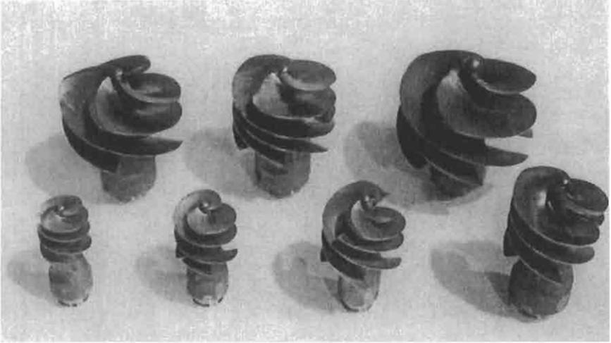
**Figure 11-7.** Inducer family for partial emission pumps (courtesy Sundstrand).
