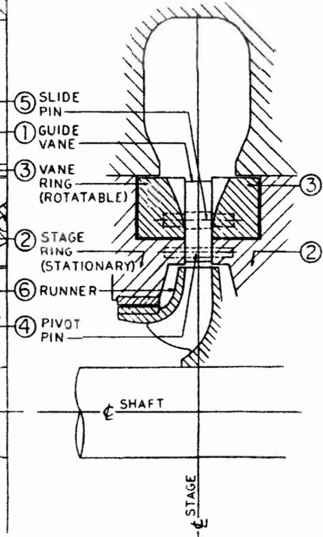
Figure 14-15. Externally adjustable guide vane assembly.
