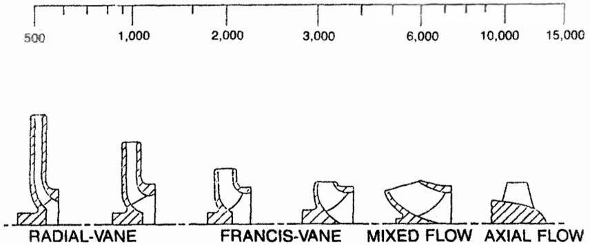
$$\text{SPECIFIC SPEED } N_s = \frac{\text{RPM } \sqrt{\text{GPM}}}{H^{3/4}}$$
