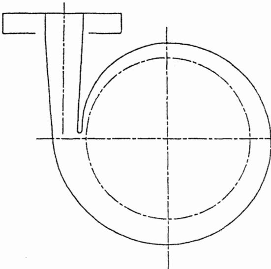
**Figure 15-10B.** Casing volute with tangential discharge nozzle.
