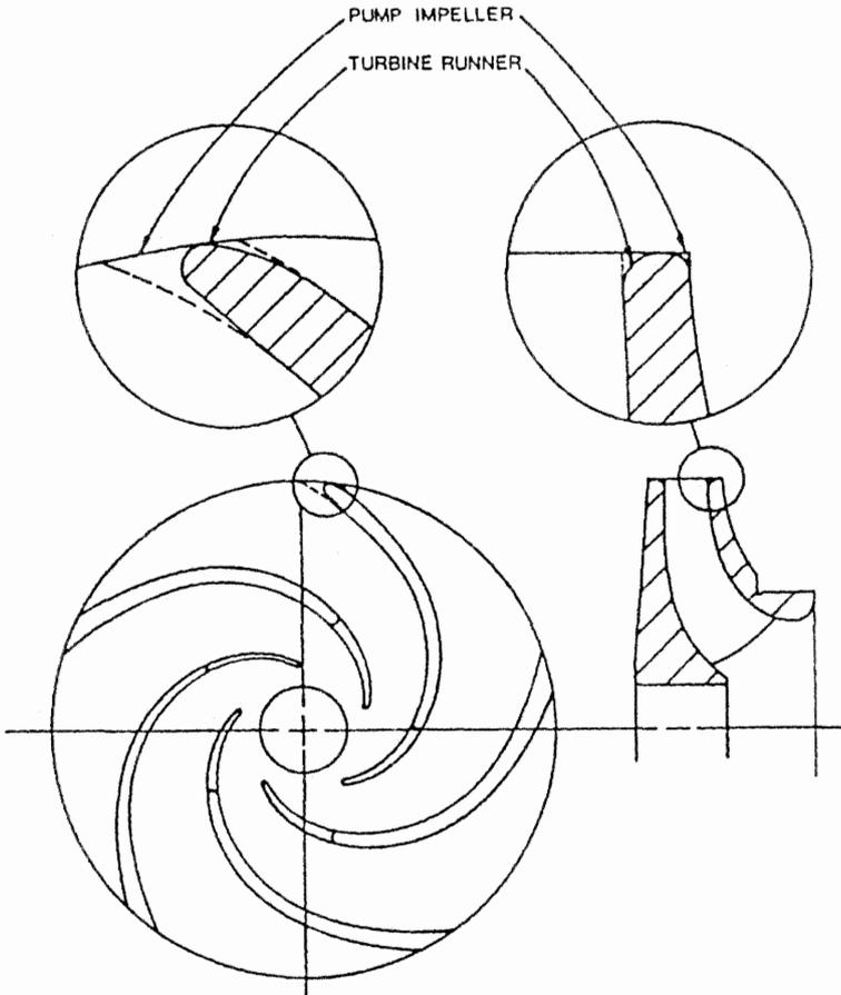
**Figure 14-6.** Rework of pump impeller for operation as an HPRT runner.
