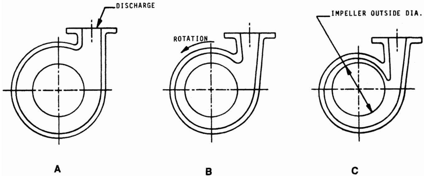
**Figure 13-4.** Casing configurations: (A) concentric volute; (B) semi-concentric volute; (C) spiral volute.
