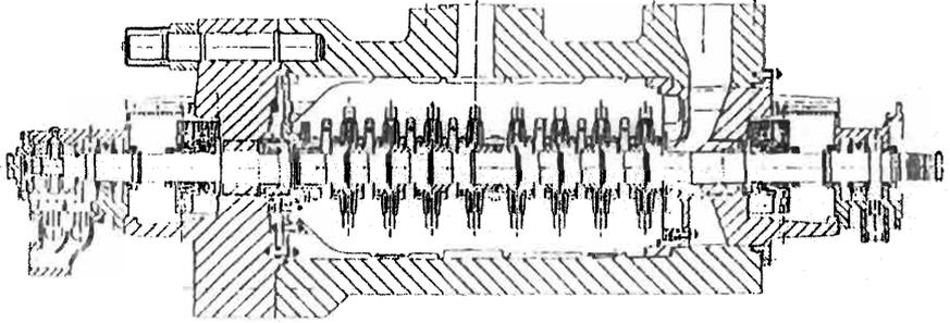
**Figure 12-6.** Water injection pump with full cartridge pullout, featuring a springplate on the high pressure end to preload the internal gasket that seals full differential pressure (courtesy BW/IP International, Inc. Pump Division, manufacturer of Byron Jackson/United™ Pumps).
