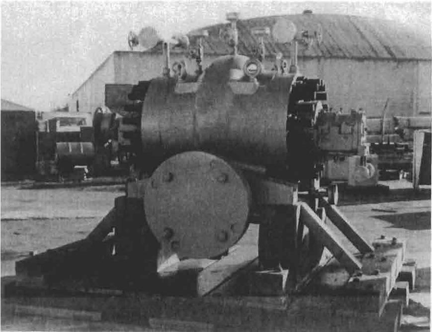
**Figure 10-35.** CO<sub>2</sub> pipeline pump (courtesy BW/IP Internal, Inc. Pump Division, manufacturer of Byron Jackson/United™ Pumps).
