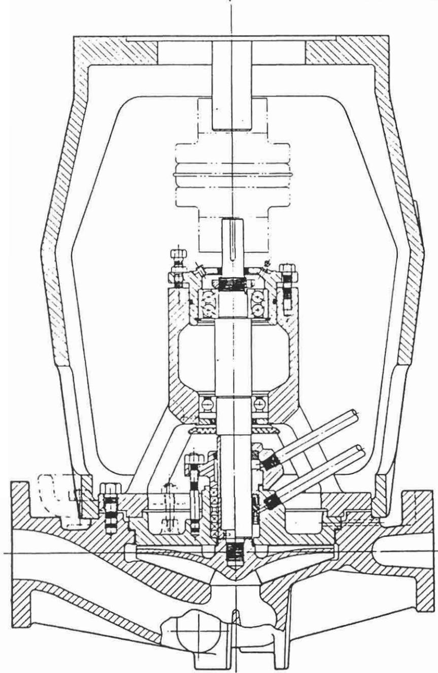
**Figure 15-8.** ANSI vertical in-line overhung single-stage pump with bearing housing (courtesy of Goulds Pumps, Inc.).
