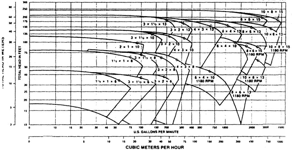
Figure 15-5. Typical 60 cycle-1800 rpm performance chart for ANSI B73.1 pumps (courtesy of Ingersoll-Rand Company).
