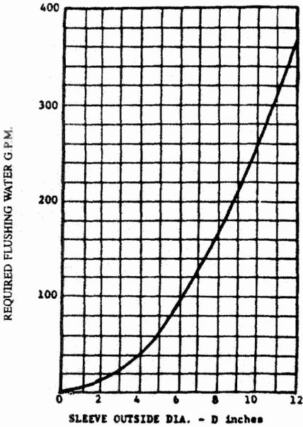
**Figure 13-6.** Approximation of flushing water requirements for “flush-type” slurry pump stuffing boxes where flush pressure is 15 psi above slurry pressure at the box. “Weep-type” stuffing boxes use about 5% of the water that “flush-types” use.
