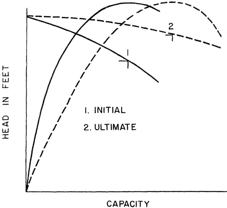
Figure 10-5. Pump performance for initial and ultimate condition.
