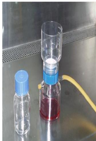
Figure 4. Media sterilization through a 0.22 \mu\text{m} membrane filter assembled in a filter holder.
