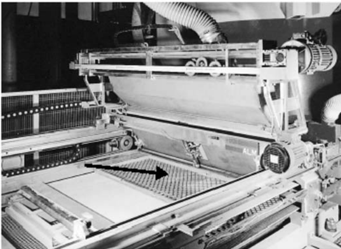
Fig. 4 Filling system with floating grating
