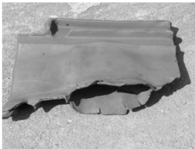
Fig. 7 Part of a roofing tile after pressing with “open” cutting lamination
