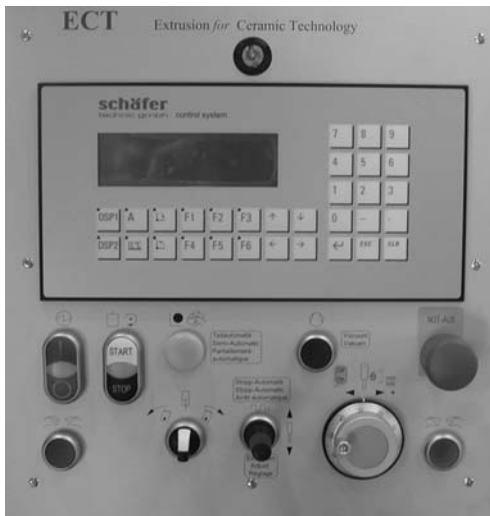
Fig. 7 Panel of a micro-processor based control system
