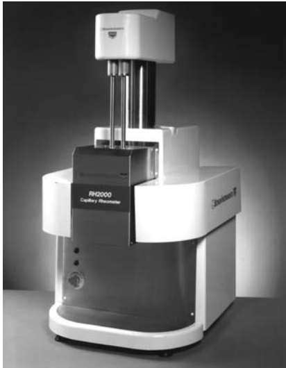
Fig. 9 Twin bore capillary rheometer (photo: Malvern)
