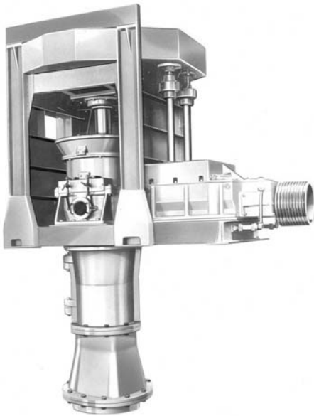
Fig. 48 Vertical extruder for stone-ware pipes
