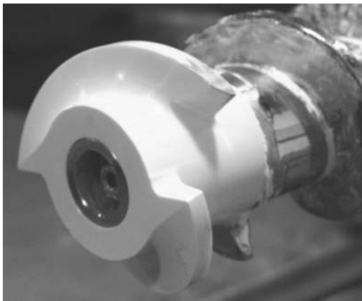
Fig. 6 Steel auger with ZrO_2 – front auger
