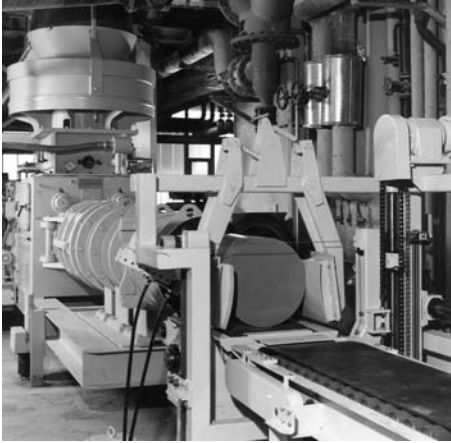
Fig. 49 Extrusion of slugs in the production of insulators
