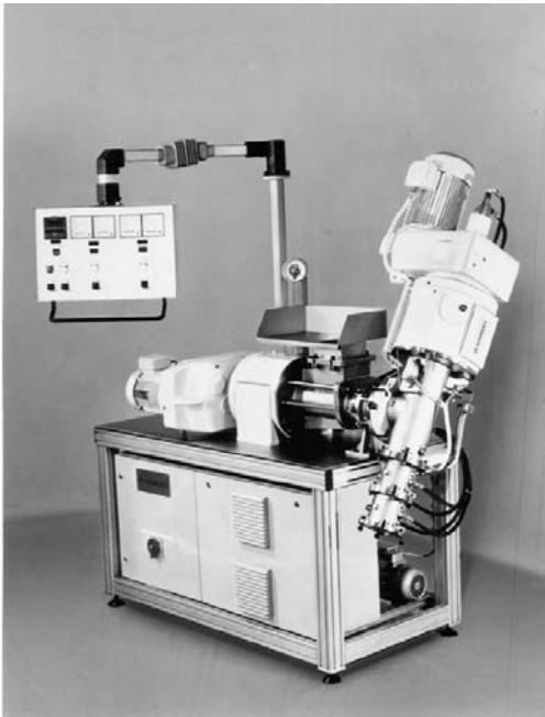
Fig. 2 Special design de-airing extruder with hinged extruder barrel
