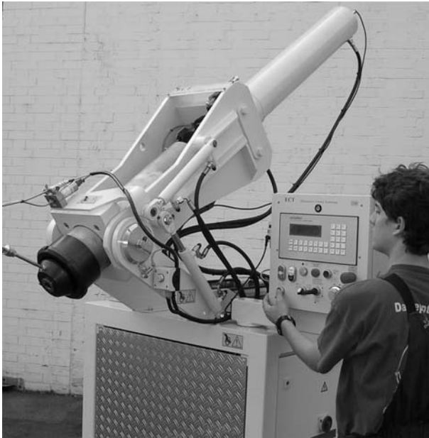
Fig. 5 140 mm piston extruder with tilting press frame
