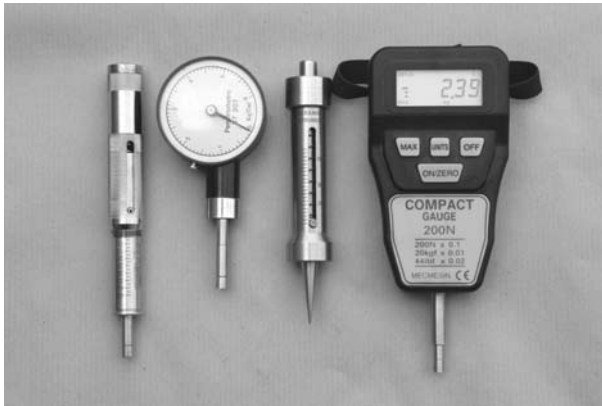
Fig. 7 Assorted penetrometer instruments (photo: ECT)
