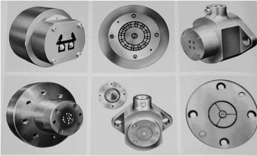
Fig. 9 A selection of combination pressure head and die assemblies for profiles and multi-channel tubes
