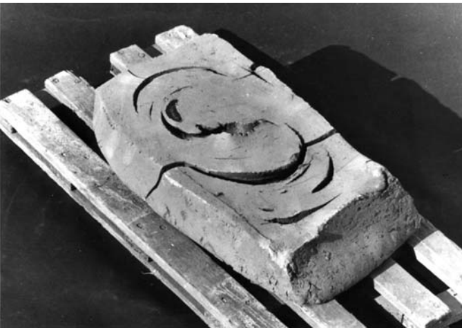
Fig. 11 Green brick showing a S-shaped crack resulting from a twin-blade point auger
