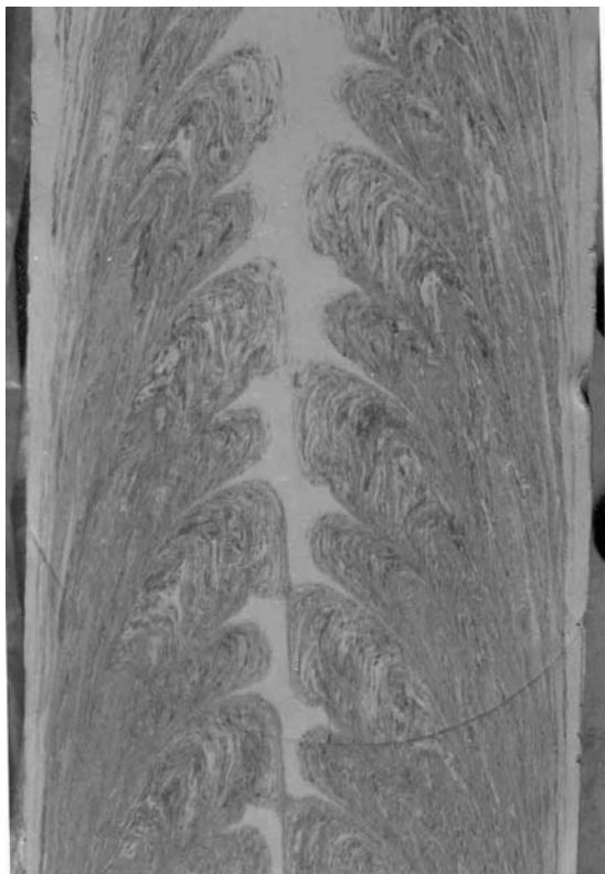
Fig. 6 Colouring test to show the laminations in a slug
