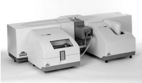
Fig. 5 Laser particle sizer (photo: Malvern)
