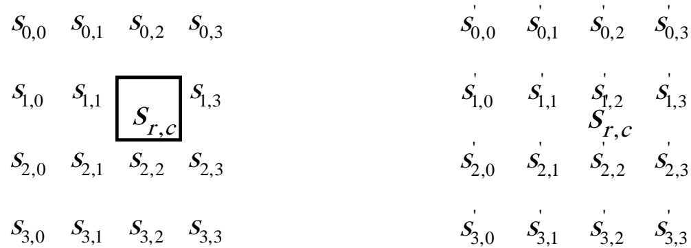
Figure 7. SubBytes() applies the S-box to each byte of the State.
