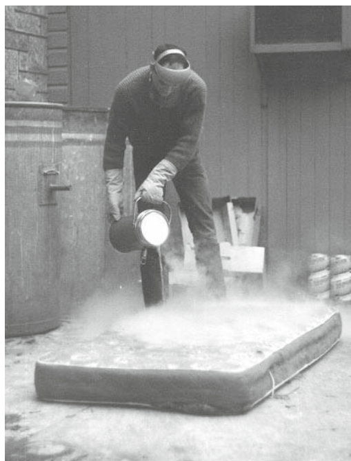
Figure 9.4 Experimental application of liquid nitrogen to a mattress for the control of dust mites.
