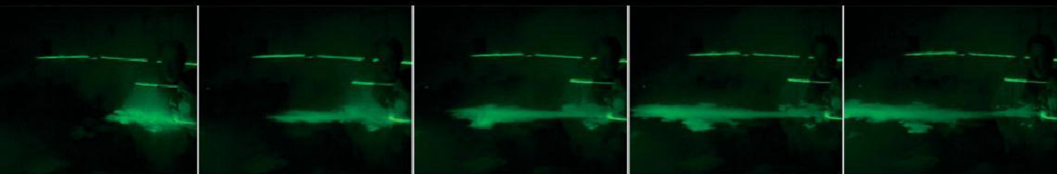
Repeating the experiment several times with different subjects demonstrated that the pattern of air movement generated by a breath has its own identifiable visual language; a central shaft flanked by two smaller eddies on either side.
