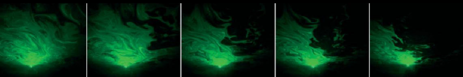
Malte Wagenfeld, Jason Parmington, Ramesh Ayyar and Ian de Gruchy, Experiments with acts of habitation: opening a door , 2007 This sequence of five images shows how the opening of a door produces a dramatic displacement of air within the interior environment.
