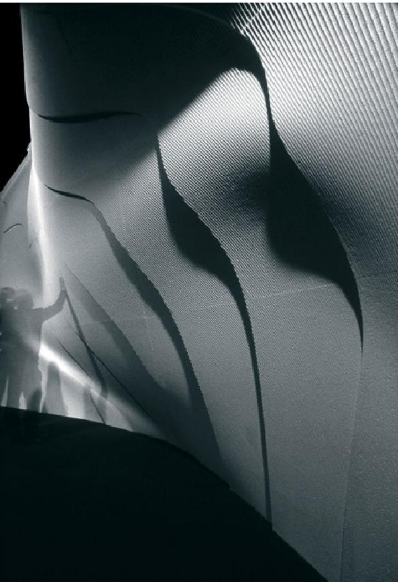
The assemblage of stacked modules reveals traits of the isoparametric machining process.
