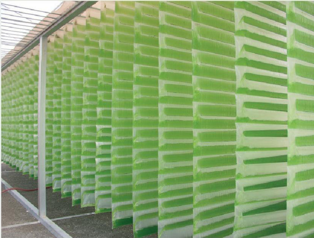
Vertigo Energy, a joint venture between Global Green Solutions and Valcent Products, is a technology for the mass production of algae by a bioreactor that grows the algae vertically for extraction of the algae oil. The oil is cost-effectively refined into a nonpolluting diesel biofuel. The algae-derived fuel is an energy-efficient, environmentally friendly replacement for fossil fuels and can be used in any diesel-powered vehicle or machinery.
