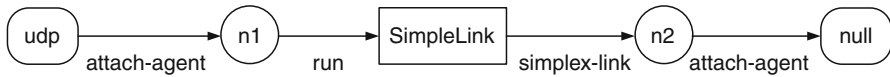
Fig. 7.4 A two-node network with a unidirectional link and the instprocs of class Simulator
