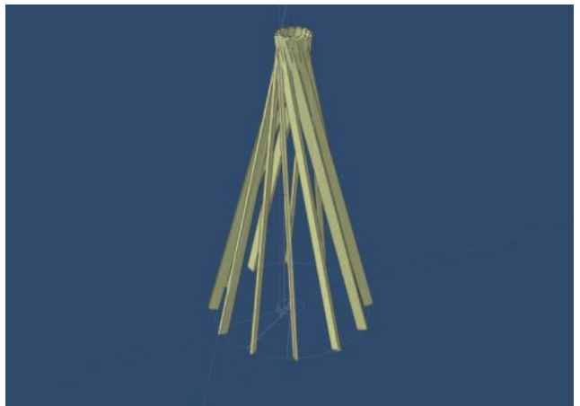
▲ 4.13 Steep RF with 12 beams. (Drawing: Chris Dunn.)
