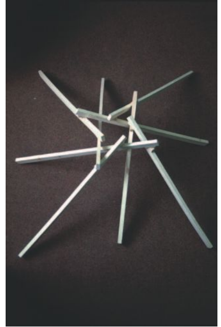
▲ 3.31 Simple RF with rotated beams.
