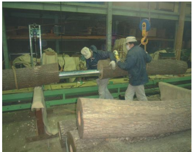
▲ 7.4 Steel core reinforcement. (Photo: Kazuhiro Ishii.)
