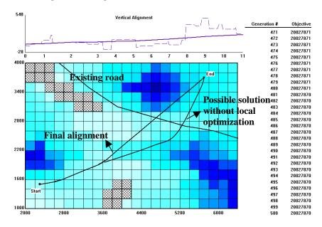
Figure 14.8: Solution in an artificial study area with 500 generations.
