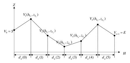
Figure 7.4: The control points on the HZ plane.
