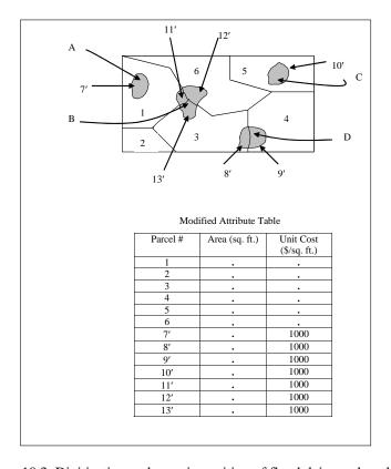
Figure 10.3: Digitization and superimposition of floodplains and wetlands.
