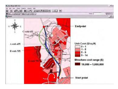
Figure 10.36: Optimized horizontal alignments for different PI's.
