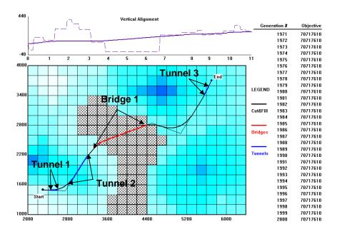
Figure 15.20: Optimized solution (scenario 5) for sensitivity analysis of tunnels.
