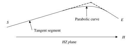
Figure 3.4: A typical vertical alignment on the HZ Plane.
