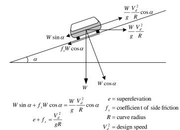
Figure 2.2: The physical relations among design speed, superelevation, coefficient of side friction, and curve radius.
