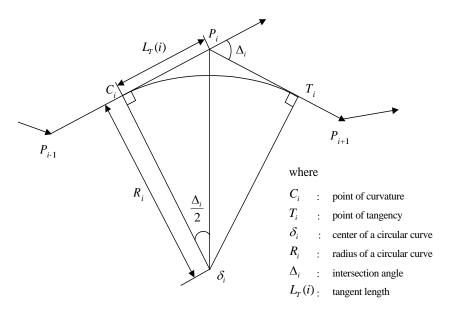
Figure 12.10: Geometric specification of a circular curve.
