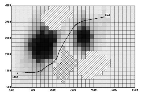
Figure 9.4: The optimized horizontal alignment for test example 1.
