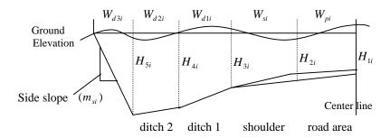
$H_{\bullet i}$  = height at each referencing point (m)  $W_{\bullet i}$  = width of each segments (m)  $m_{\circ i}$  = side slope (decimal)
