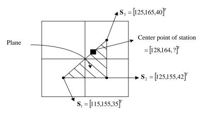
Figure 12.8: Surrounding vectors of station B's center point.
