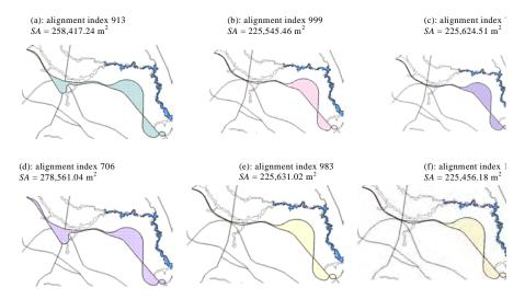
Figure 10.44: Intervening area of significantly different alignments.
