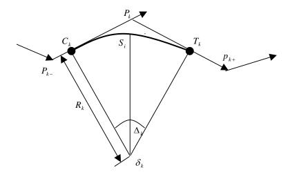
where  $\delta_k$  = center of  $k^{th}$  circular point  $P_k$  =  $k^{th}$  point of intersection  $R_k$  = radius of  $k^{th}$  circular curve  $\Delta_k$  = angle of  $k^{th}$  circular curve
