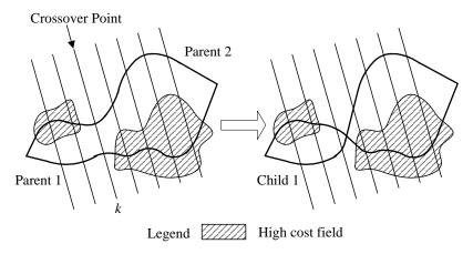
Figure 5.5: An example of a simple crossover operator.
