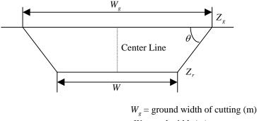
W = road width (m)  $z_g = \text{ground elevation of center line (m)}$   $z_r = \text{road elevation of center line (m)}$  $\theta = \text{side slope (degree)}$
