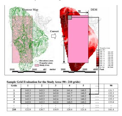
Figure 10.34: Ground elevation of the study area in Brookeville.
