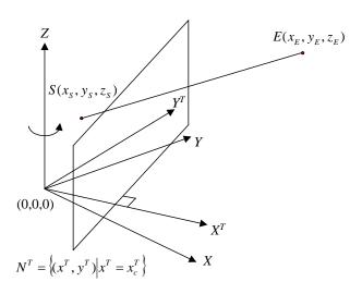
Figure 3.6: The coordinate transformation from XYZ to  $X^TY^TZ$ .
