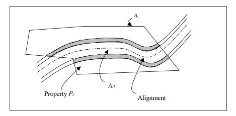
Figure 10.12: A property intersected by a highway alignment.
