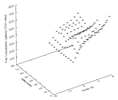
Figure 4.20: Fuel consumption data plots: 3-S2 diesel truck.
