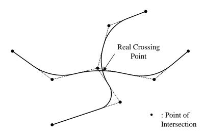
Figure 12.9: Points of intersections (PI's) and final crossing point deviating from its original PI.
