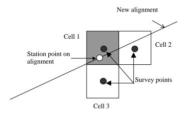
Figure 13.1: A general case for obtaining ground elevations.
