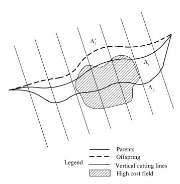
Figure 5.8: An example of a heuristic crossover operator.
