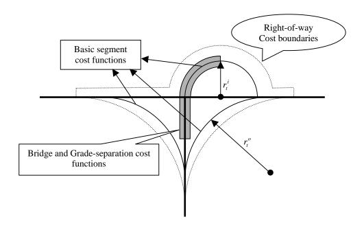
Figure 12.31: Centerlines of a typical trumpet interchange, major design criteria and separated parts for each cost function.
