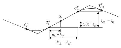
Figure 7.11: Station point on a tangent section of the vertical alignment.
