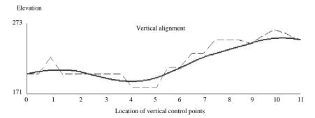
Figure 9.25: The optimized vertical alignment found by Model 3 for test example 2.
