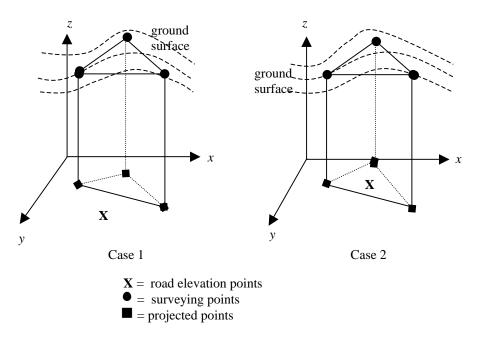
Figure 12.5: Two possible cases when projecting ground elevations onto *xy* plane.
