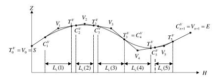
Figure 7.9: An example of vertical alignments.
