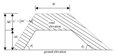
Figure 12.28: Typical cross section with insufficient vertical clearances.
