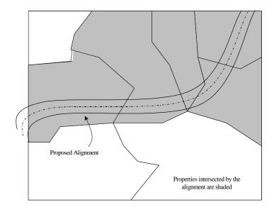
Figure 10.10: Properties intersected by an alignment.
