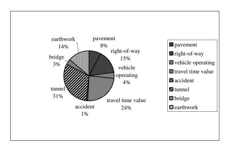
Figure 15.8: Cost breakdown for the new alignment in Figure 15.6.
