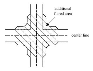
Figure 12.12: A typical four-legged intersection.
