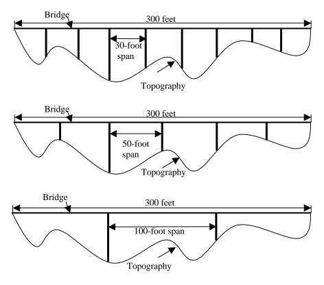
Figure 12.24: Equally spaced piers with varying spans.
