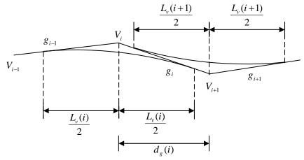
Figure 7.5: An example of discontinuity in vertical curve.
