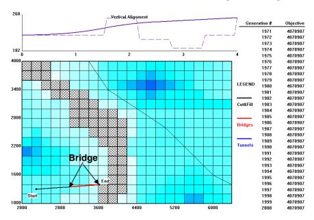
Figure 15.43: Optimized solution for segment 1 under scenario 3.
