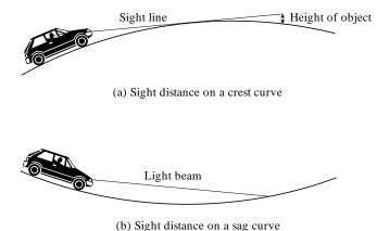
Figure 2.4: Geometry of vertical sight distance.
