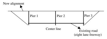
Figure 13.4: An example freeway overpass with three piers.
