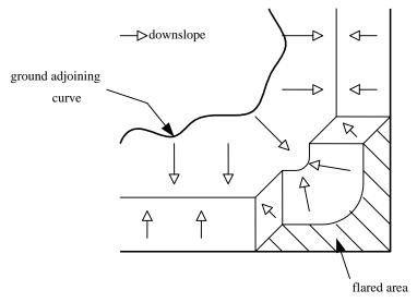
Figure 12.14: Quadrant of a typical fill intersection.
