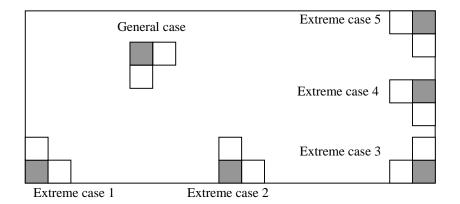
Figure 13.2: Extreme cases when choosing two adjacent cells for planar Interpolation.
