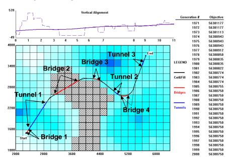
Figure 15.19: Optimized solution (scenario 4) for sensitivity analysis of tunnels.
