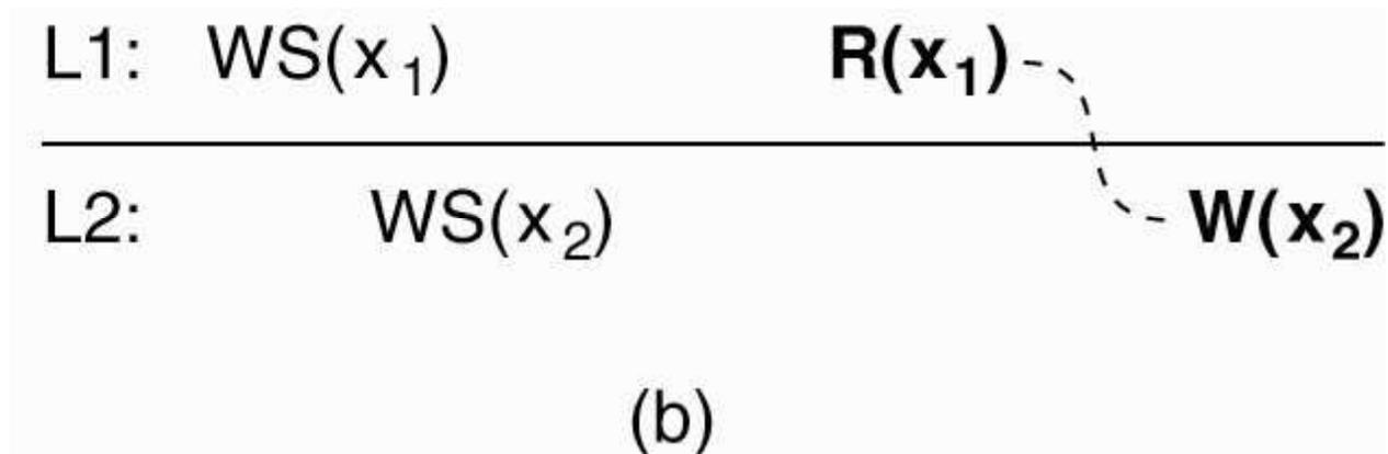
Figure 7-15. (b) A data store that does not provide writes-follow-reads consistency.
