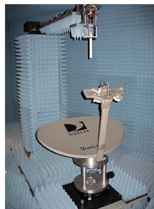
Figure 29. DirecTV multifeed offset parabolic reflector antenna in plane-polar near-field measurement facility at UCLA.
