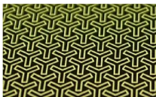
Figure 20. Example of a dichroic FSS, from www.q-par.com .
