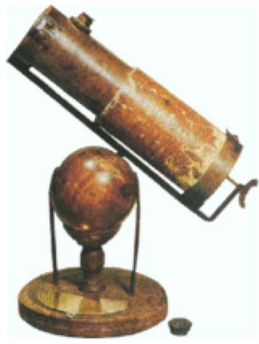
Figure 4. Newton's parabolic reflector optical telescope, 1672.
