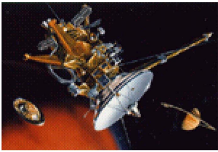
Figure 19. Cassini spacecraft 4-m antenna with S/X/Ku/Ka-band FSS.
