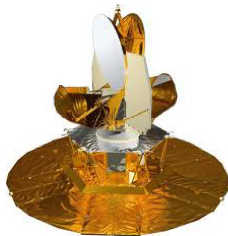
Figure 18. WMAP doubly shaped Gregorian reflector antennas.
