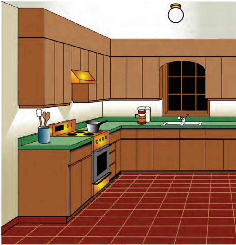
FIGURE 20.10 A good balance between ambient and task lighting can be had by combining under-cabinet fixtures with fixtures mounted on the ceiling.
