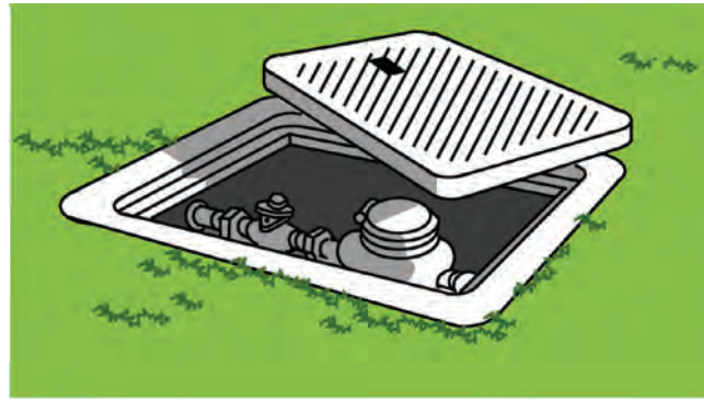
FIGURE 16.1 The water meter and main shutoff valve usually are located in the front yard near the property line.
