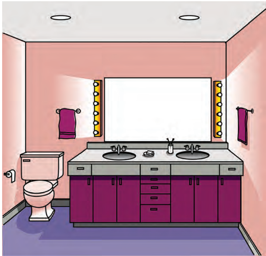
FIGURE 20.16 Fixtures mounted at both sides of a mirror are the most effective way to spread light where it is wanted on the user's face. This may provide all of the light required in a small bath. Larger baths may require additional fixtures for task or ambient lighting.
