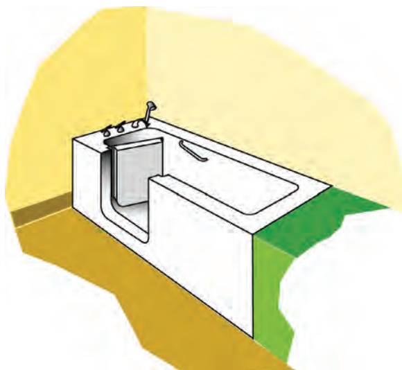
FIGURE 18.5 Tubs equipped with doors in the side make it easier for persons with special needs to get in and out of the fixture.
