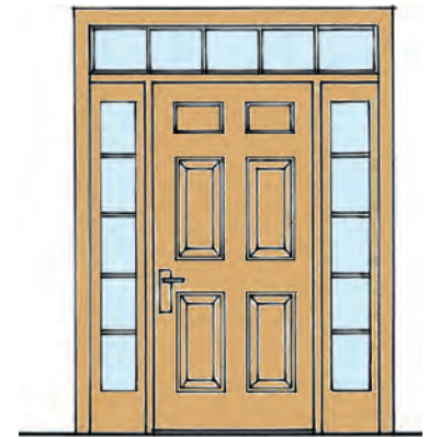
FIGURE 9.4 An entrance system combines one or more doors, flanking sidelights, and transom windows into a single frame. Many combinations and styles are possible.
