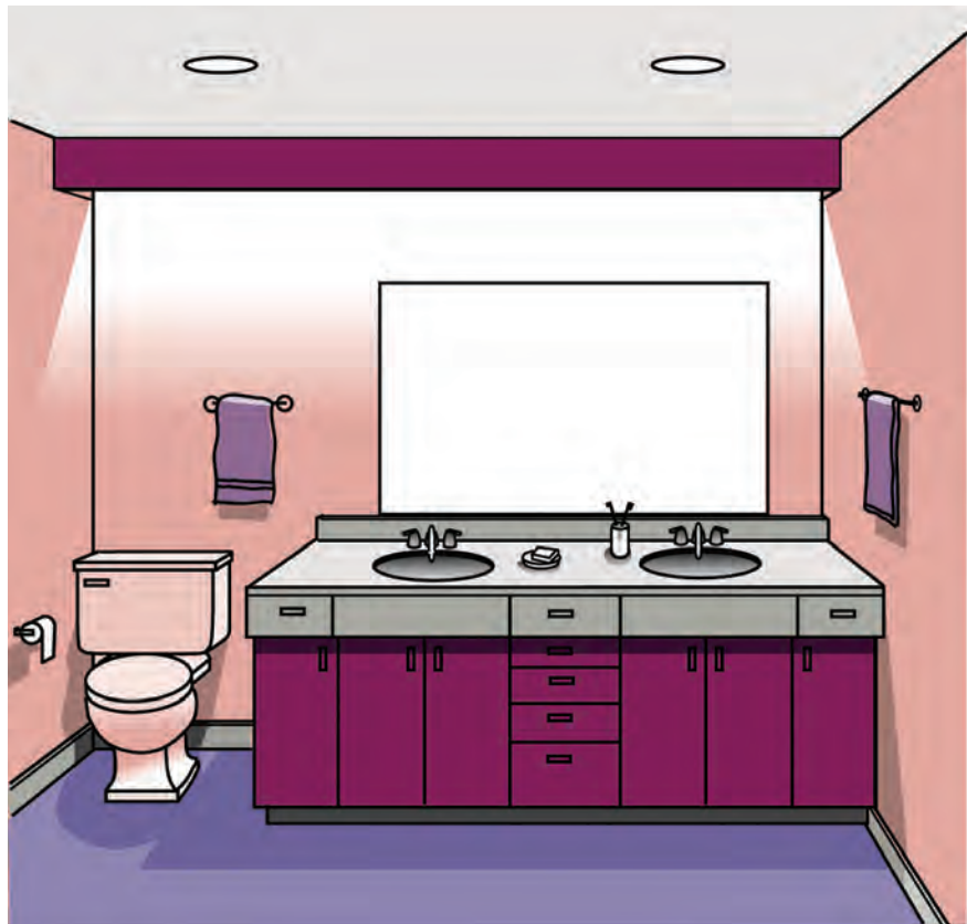
FIGURE 20.17 Task lighting at a vanity can be provided by a fluorescent strip fixture mounted behind a valance.
