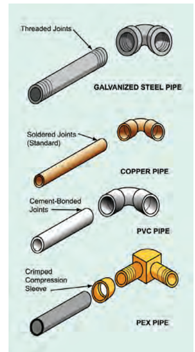
FIGURE 16.5 Four materials make up the bulk of most residential water supply piping. Copper still reigns as the most popular for new construction, while PEX is gaining due to its flexibility and ease of installation.
