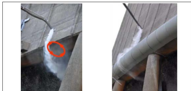
Figure 3: Smoke test of the air inflow conditions at the cooling tower shell at Leibstadt (left side with normal air inflow – right side with improved air inflow using a simplified spoiler)
