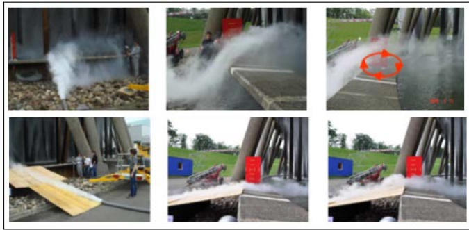
Figure 2: Smoke test of the air inflow conditions at the cooling tower basin of the Leibstadt (upper photos show normal air inflow – lower photos demonstrate improved air inflow using a simple wooden plank)
