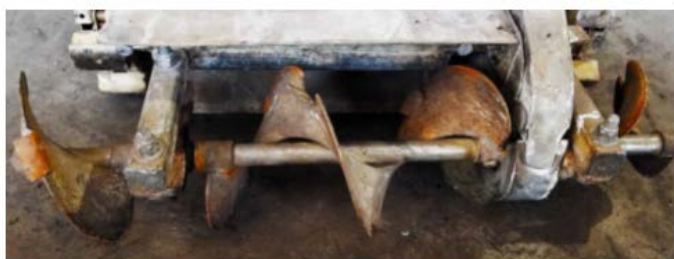
Figure 4 - Auger at front of robot
