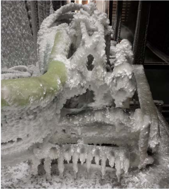
Figure 10 – Robot Exposed to Extreme Cold during use
