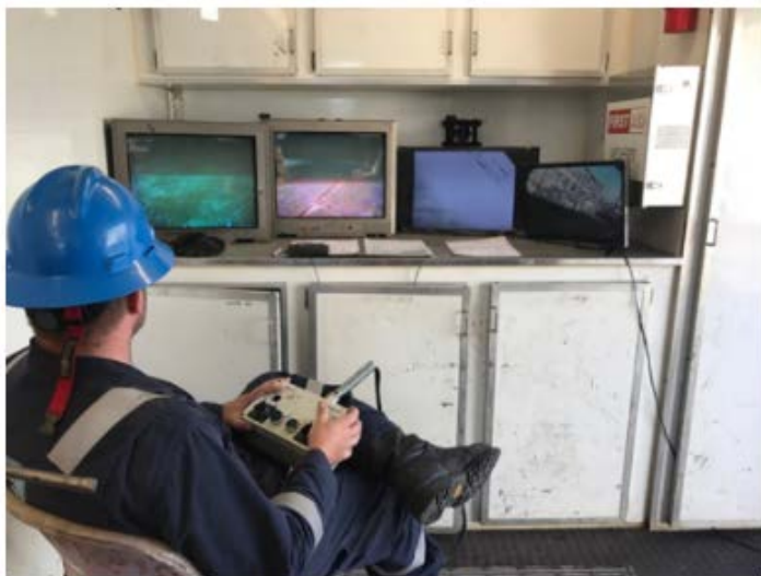
Figure 3 - Online robotic tank cleaning operator
