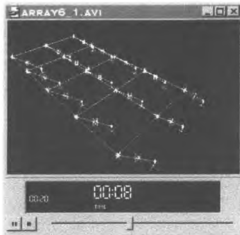
Fig. 9.25 Snapshot of video clip showing response of the system to the 1979 Imperial Valley as recorded at the El Centro Array #6 recording station.
