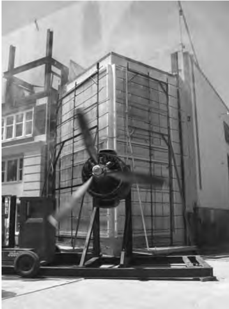
9.3 Airplane engine is used to create dynamic pressure for the wind-driven rain test.
