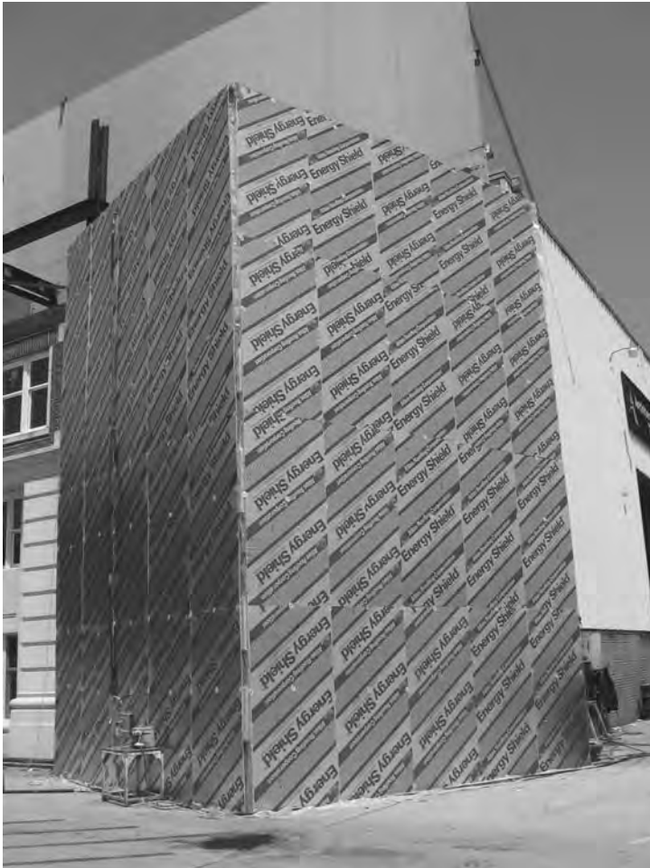
9.6 Three-story (32 feet) insulated enclosure is used for thermal cycling of a large preconstruction mock-up with outside 90° corner condition.
