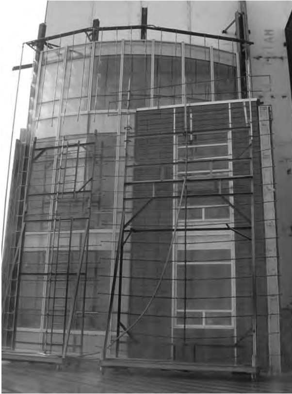
9.2 Static water resistance testing on a full-scale preconstruction mock-up. Water is applied to the exterior face at the rate of 5.0 US gallons per square foot per hour.
