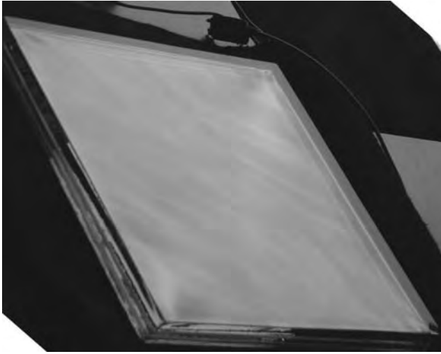
6.5 Visible quench pattern in laminated heat-treated glass reflecting a uniform blue sky.
