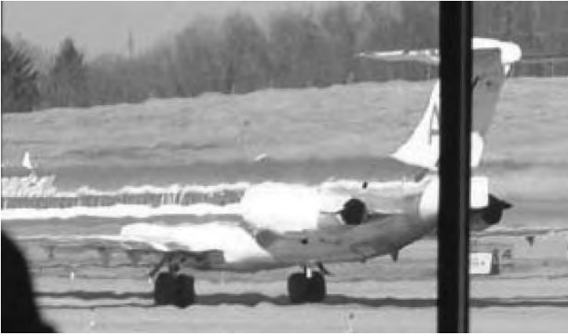
6.6 Example of transmission distortion caused by laminating plies of heat-treated glass.
