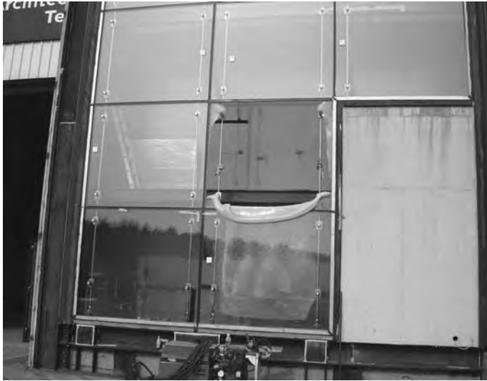
9.8 Glazing failure in performance during structural testing. Notice the 'wet blanket' effect of a fully tempered laminated glass unit.
