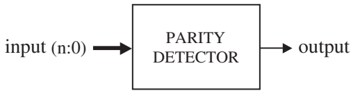
Figure 4.3 Generic parity detector of example 4.2.
